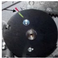
Figure 2 - Index Mark on Z-Index Flag
