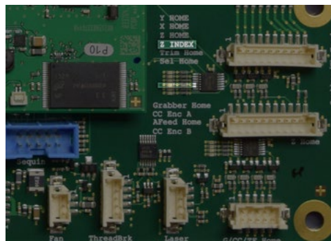
Figure 5 - Z-Index LED (Location D50)
