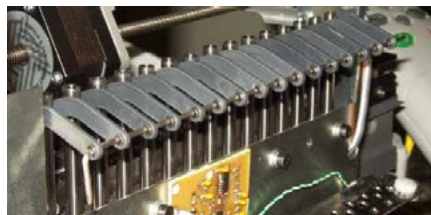
Figure 2 Wire Installed Through Take Up Levers
