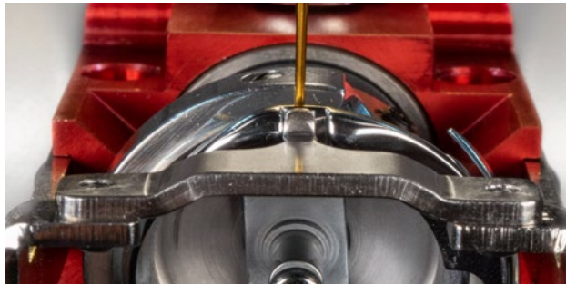
Figure 4 – Hook Support Position Left-to-Right
