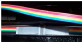
Figure 2 - Retaining Clip in Channel of Y-Home Flag
