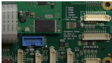
Figure 4 - Grabber/Thread Feed Motor Connection at PCB
