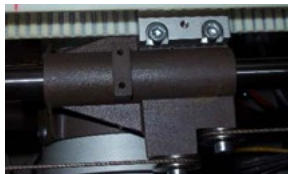
Figure 2 - Cable Bracket Removal
