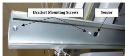
Figure 2 - X-Home Sensor and Mounting Screws
