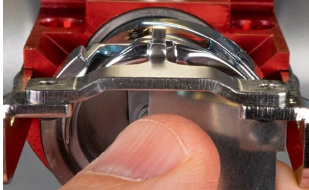
Figure 5 – Retaining Finger Gauge Usage
