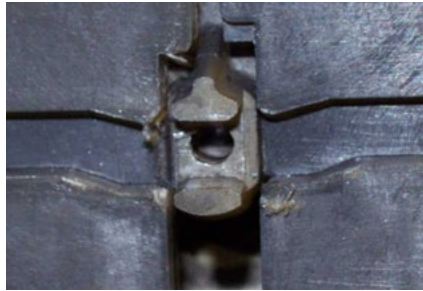
Figure 1 - Reciprocator Drive Groove at "Head Up" Position
