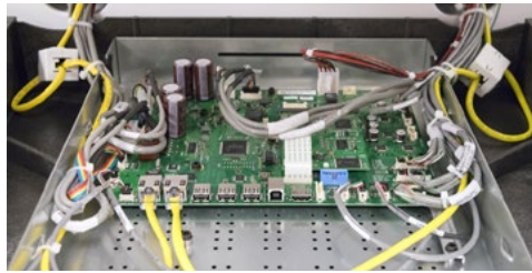
Figure 1 - Main PCB Installed
