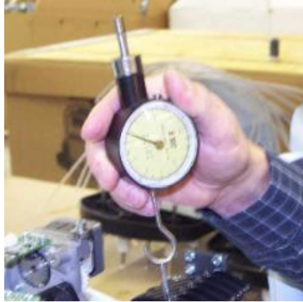
Figure 1: Measurement of Take-Up Lever Pull Force
