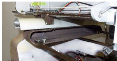
Figure 1 - X-Beam and Carriage Installed on Machine
