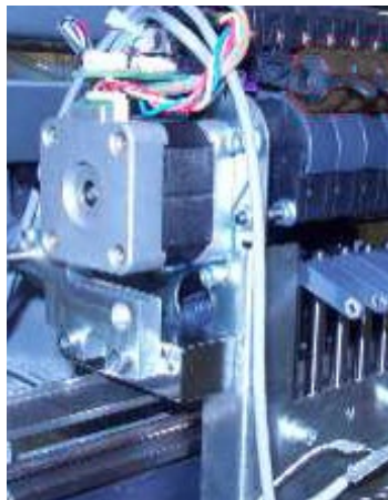
Figure 4 - Routing of Harness to Top of Needlecase
