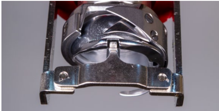
Figure 2 – Rotary Hook Basket Notch
