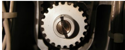
Figure 3 - Lower Z-Shaft Drive Pulley
