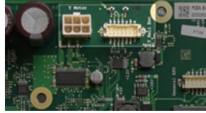
Figure 2 - Y-Motor Connections at PCB
