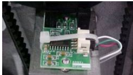
Figure 2 - Cable Tie Around PCB
