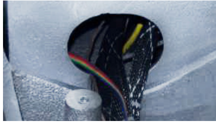
Figure 3 - Left Lower Arm Access Hole
