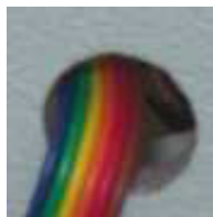
Figure 3 - X/Y Home Harness Access Hole
