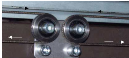
Figure 6 - Center Beam Cable Pulley (Arrows indicate direction of cable to the front)
