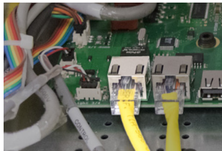
Figure 3 - Ethernet Connector Location on Main PCB ("Eth")
