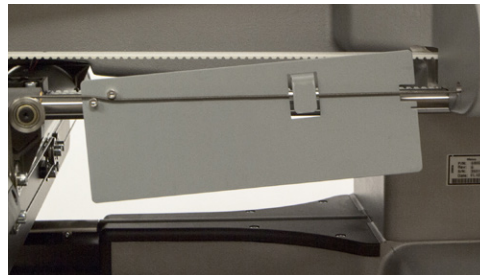
Figure 5: Positioning the X-Cable Tension Gauge
