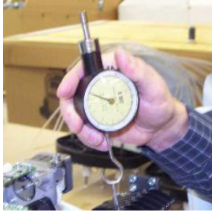
Figure 1: Measurement of Take-Up Lever Pull Force
