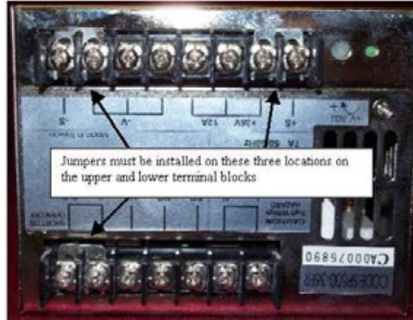
Figure 2 - Power Supply Unit Terminal Jumpers
