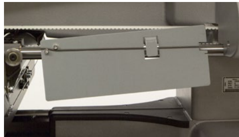
Figure 5: Positioning the X-Cable Tension Gauge
