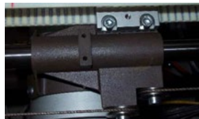
Figure 2 - Cable Bracket Removal
