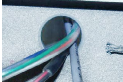
Figure 2 - Right Upper Arm Access Hole
