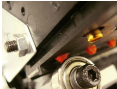
Figure 7 - Thread Feeder Clicker
