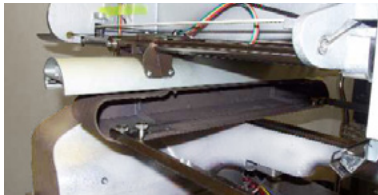
Figure 1 - X-Beam and Carriage Installed on Machine
