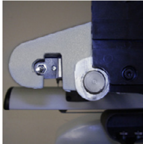
Figure 10 - Cable Tensioning Bracket (Left side of machine)
