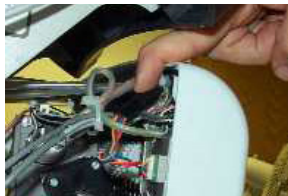
Figure 2 - Thread Feed Motor Lead
