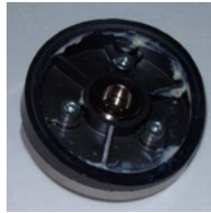
Figure 3 - Screws On Back of Take-Up Lever Cam
