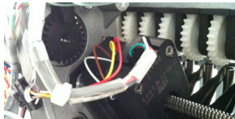
Figure 1 - Color Change Harness Connection to Motor
