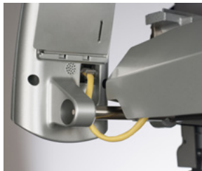
Figure 2 - Keyboard Harness Connection
