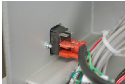
Figure 2 - Power Switch Interface Harness Wiring to Switch
