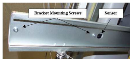
Figure 2 - X-Home Sensor and Mounting Screws
