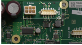
Figure 2 - Y-Motor Connections at PCB
