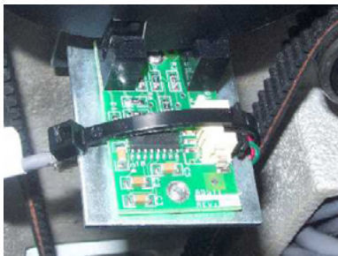
Figure 1 - Connection to Z-Index PCB
