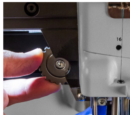
Figure 2 - Presser Foot Height Adjustment Eccentric
