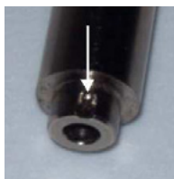
Figure 6 - Alignment Groove in Z-Shaft
