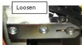
Figure 2 - Right Take Up Lever Bar Mounting Block
