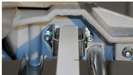
Figure 3 - Y-Drive Timing Belt Adjusting Screws
