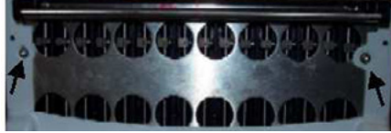
Figure 2 - Needlecase Access Cover Removed
