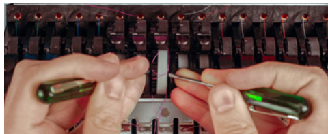
Figure 2 - Prying Thread Feeder Roller Loose
