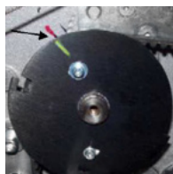
Figure 2 - Index Mark on Z-Index Flag
