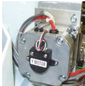
Figure 3 - Harnessing Routed Under Y-Motor
