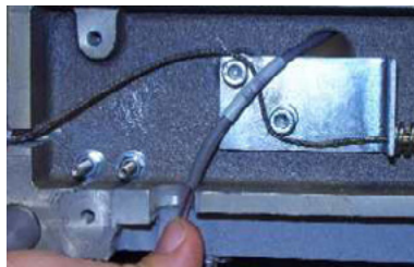
Figure 1 - Left LED Cluster Harness
