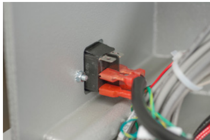
Figure 2 - Power Switch Interface Harness Wiring to Switch
