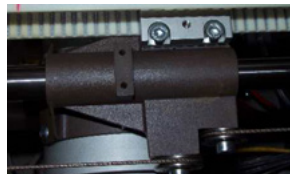
Figure 2 - Cable Bracket Removal
