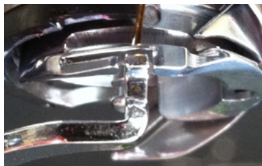
Figure 2 – Rotary Hook Basket Notch
