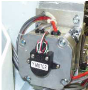
Figure 3 - Harnessing Routed Under Y-Motor
