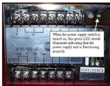
Figure 3 - Power Supply Indicator LED
