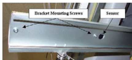
Figure 2 - X-Home Sensor and Mounting Screws
