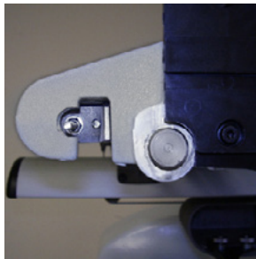
Figure 10 - Cable Tensioning Bracket (Left side of machine)
