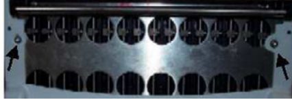
Figure 2 - Needlecase Access Cover Removed
