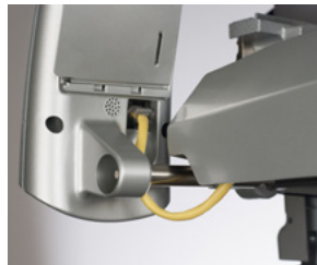
Figure 1 - User Interface Harness Connection
