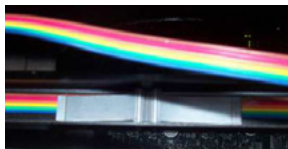
Figure 2 - Retaining Clip in Channel of Y-Home Flag
