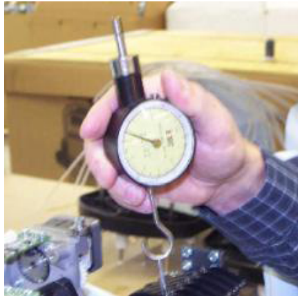
Figure 1: Measurement of Take-Up Lever Pull Force
