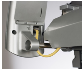
Figure 2 - Keyboard Harness Connection
