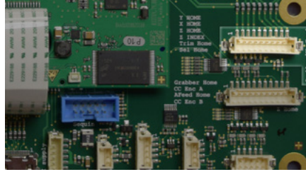
Figure 4 - Grabber/Thread Feed Motor Connection at PCB
