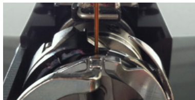
Figure 4 – Hook Support Position Left-to-Right
