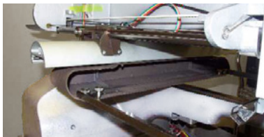
Figure 1 - X-Beam and Carriage Installed on Machine
