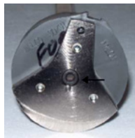
Figure 2 - Remove Center Screw
