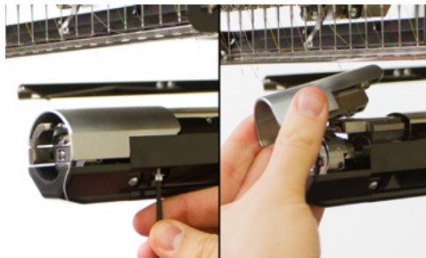
Figure 2 – Needle Plate Screws
