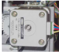
Figure 1 - Thread Feeder Stepper Motor
