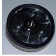
Figure 3 - Screws On Back of Take-Up Lever Cam
