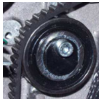
Figure 1 - Z-Belt Idler Pulley
