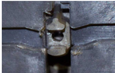
Figure 2 - Reciprocator at "Head Up" Position
