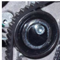
Figure 3 - Z-Belt Idler Pulley
