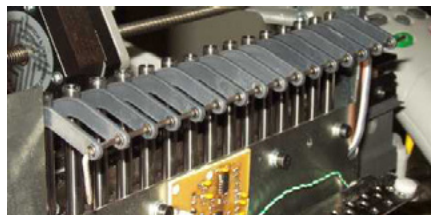
Figure 2 Wire Installed Through Take Up Levers
