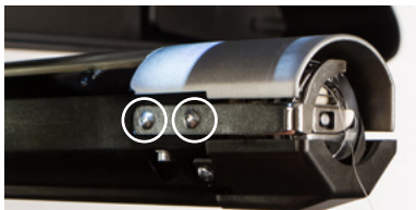
Figure 1 – Hook Support Screws
