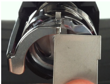
Figure 5 – Retaining Finger Gauge Usage
