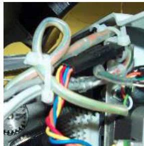
Figure 5 - Harness Tie at Top Left of Needlecase Assembly
