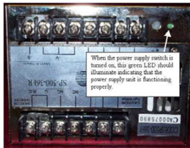
Figure 3 - Power Supply Indicator LED
