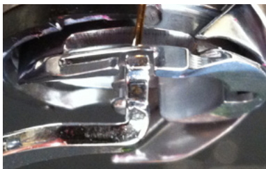
Figure 2 – Rotary Hook Basket Notch
