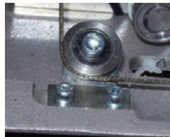
Figure 8 - Left Rear Cable Pulley
