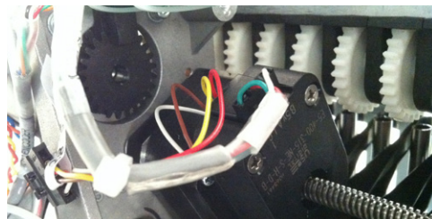
Figure 1 - Color Change Harness Connection to Motor
