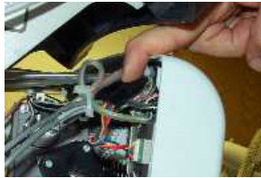
Figure 2 - Thread Feed Motor Lead
