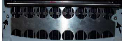
Figure 2 - Needlecase Access Cover Removed
