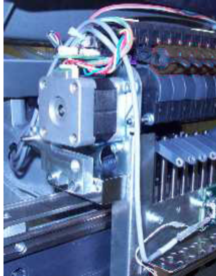
Figure 4 - Routing of Harness to Top of Needlecase
