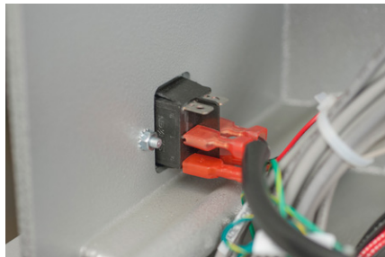
Figure 2 - Power Switch Interface Harness Wiring to Switch
