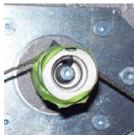
Figure 2 - Wrap Tape Around X-Drive Pulley
