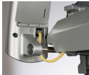
Figure 1 - User Interface Harness Connection
