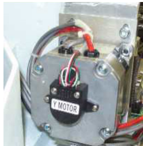
Figure 3 - Harnessing Routed Under Y-Motor
