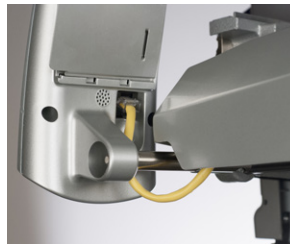
Figure 2 - Keyboard Harness Connection
