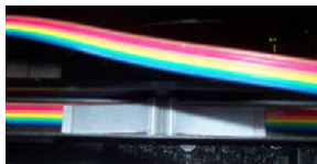
Figure 2 - Retaining Clip in Channel of Y-Home Flag
