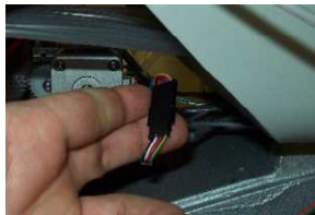
Figure 1 - Grabber Motor Lead
