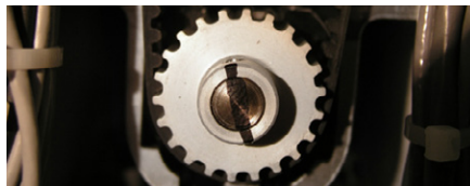
Figure 3 - Lower Z-Shaft Drive Pulley
