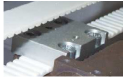
Figure 3 - Right Y-Drive Timing Belt Clamp
