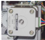
Figure 1 - Thread Feeder Stepper Motor
