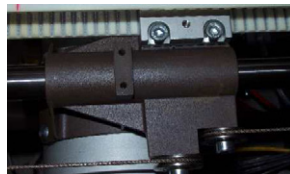
Figure 2 - Cable Bracket Removal
