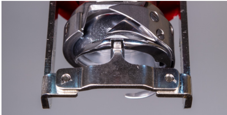
Figure 2 – Rotary Hook Basket Notch
