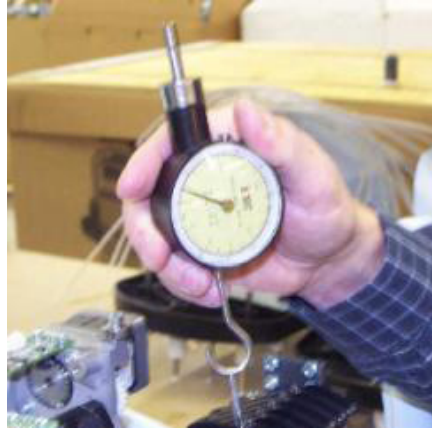
Figure 1: Measurement of Take-Up Lever Pull Force
