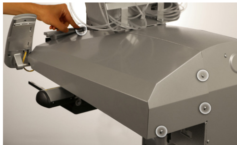
Figure 2: Removing the right cover
