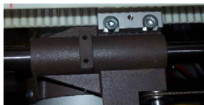
Figure 1 - Bearing Block Assemblies
