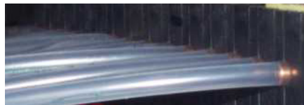
Figure 2 - Thread Tubes Connected to Thread Feeder Assembly
