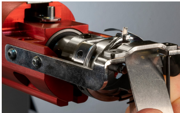
Figure 3 – Hook Support Adjustment
