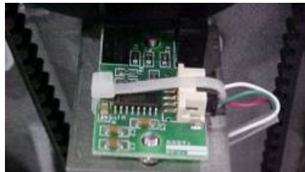
Figure 2 - Cable Tie Around PCB
