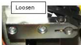
Figure 2 - Right Take Up Lever Bar Mounting Block
