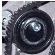
Figure 3 - Z-Belt Idler Pulley
