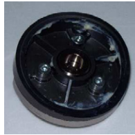
Figure 3 - Screws On Back of Take-Up Lever Cam
