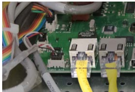
Figure 3 - Ethernet Connector Location on Main PCB ("Eth")
