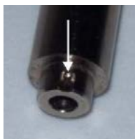
Figure 6 - Alignment Groove in Z-Shaft
