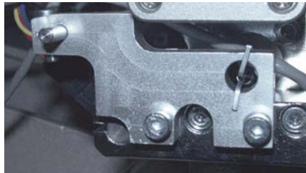
Figure 1- Left Color Change Spindle Mounting Bracket
