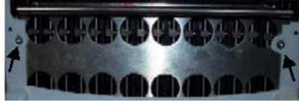
Figure 2 - Needlecase Access Cover Removed
