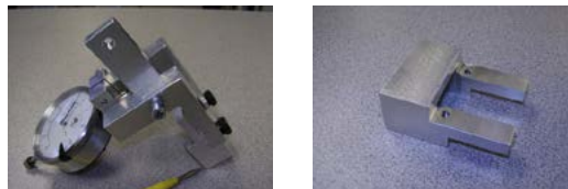
Figure 2 - Adaptor and Dial Indicator
