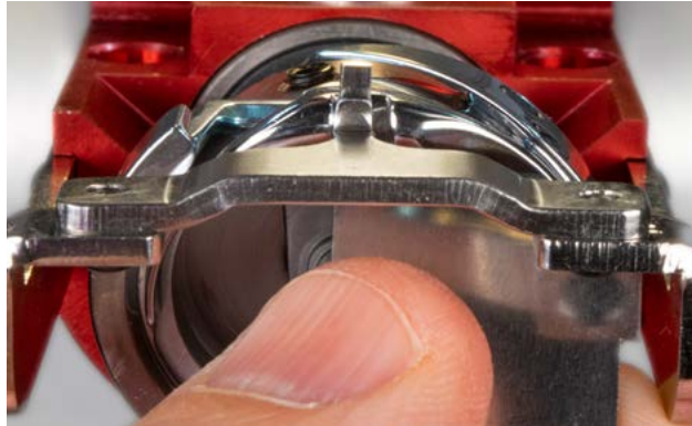
Figure 5 – Retaining Finger Gauge Usage
