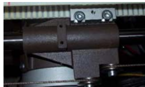
Figure 2 - Cable Bracket Removal
