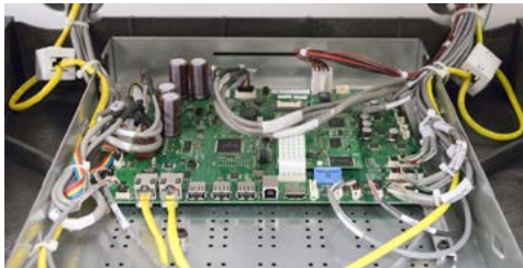
Figure 1 - Main PCB Installed
