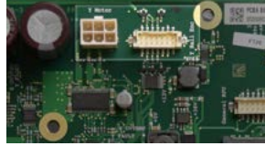
Figure 2 - Y-Motor Connections at PCB
