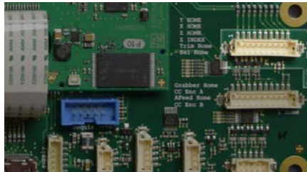
Figure 4 - Grabber/Thread Feed Motor Connection at PCB
