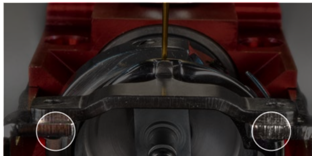
Figure 1 – Screws toward front
