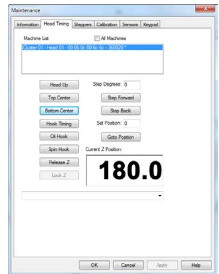
Figure 1 - Head Timing Menu
