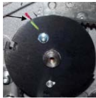
Figure 2 - Index Mark on Z-Index Flag
