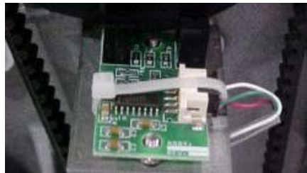
Figure 2 - Cable Tie Around PCB
