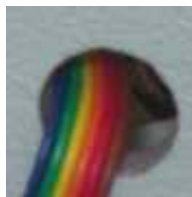
Figure 3 - X/Y Home Harness Access Hole
