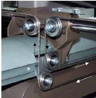
Figure 5 - Right Beam Cable Pulleys (Arrows indicate direction of cable to the front)
