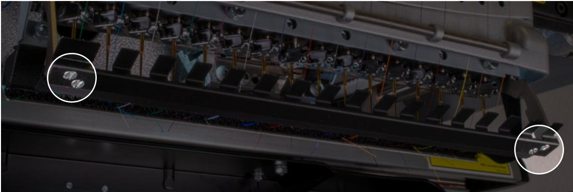
Figure 1 - Grabber Blade (bottom view)
