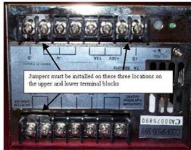
Figure 2 - Power Supply Unit Terminal Jumpers
