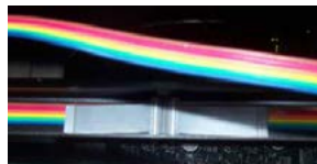
Figure 2 - Retaining Clip in Channel of Y-Home Flag
