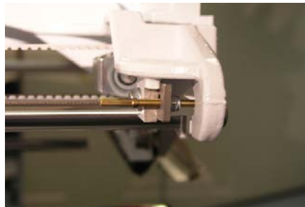
Figure 3 - X-Cable Tensioning Screw
