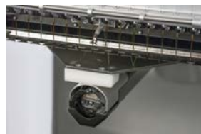
Figure 2 - X/Y-Home Fixture in Needle Plate Hole
