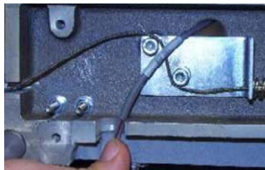
Figure 1 - Left LED Cluster Harness
