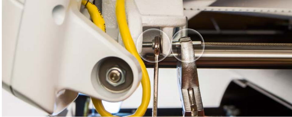
Figure 7:X-Cable Tension Adjustment
