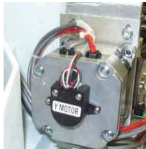
Figure 3 - Harnessing Routed Under Y-Motor
