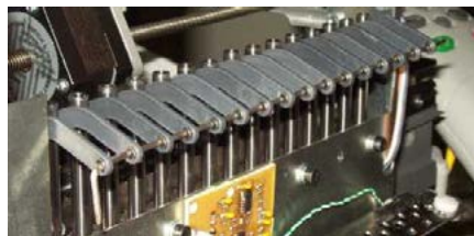
Figure 2 Wire Installed Through Take Up Levers
