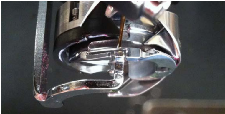
Figure 2 – Rotary Hook Basket Notch
