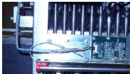
Figure 1 - Threadbreak Harness Connected to Sensor PCB
