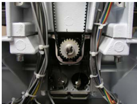
Figure 2 - Bobbin Shaft Timing Pulley (Rear)
