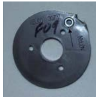
Figure 4 - Remove Hex Nut
