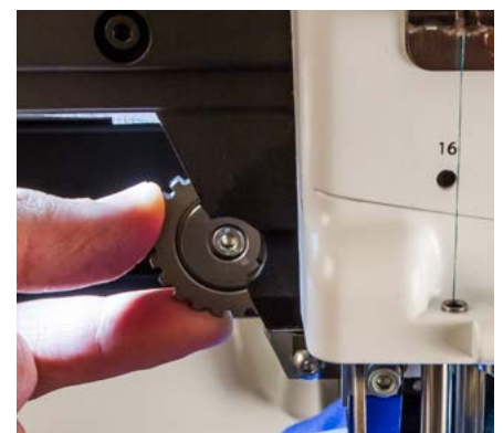
Figure 2 - Presser Foot Height Adjustment Eccentric
