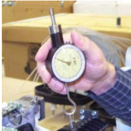
Figure 1: Measurement of Take-Up Lever Pull Force
