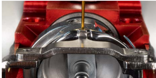
Figure 4 – Hook Support Position Left-to-Right
