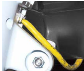
Figure 2 - Keyboard Harness Connection
