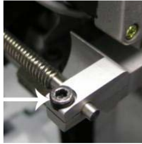
Figure 3 - Loosen Top Screw
