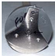
Figure 2 - Remove Center Screw
