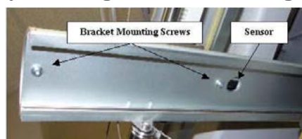
Figure 2 - X-Home Sensor and Mounting Screws
