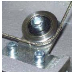
Figure 4 - Right Rear Pulley Close Up
