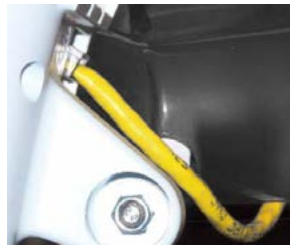
Figure 1 - User Interface Harness Connection
