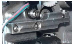
Figure 2 - Right Color Change Spindle Mounting Bracket
