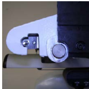
Figure 10 - Cable Tensioning Bracket (Left side of machine)
