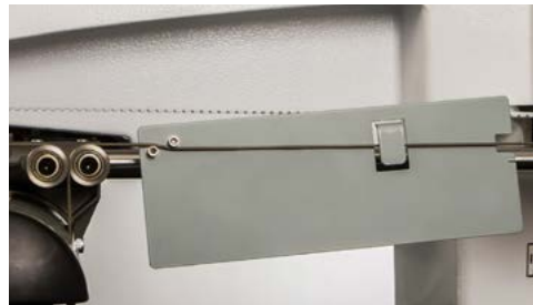
Figure 5: Positioning the X-Cable Tension Gauge
