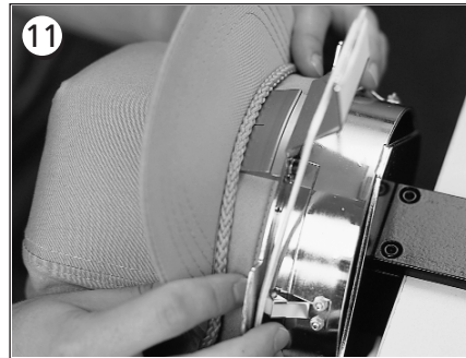
Now place the cap on the cap frame. The sweatband should be under the locator, and the brim should be centered and pointing up.
