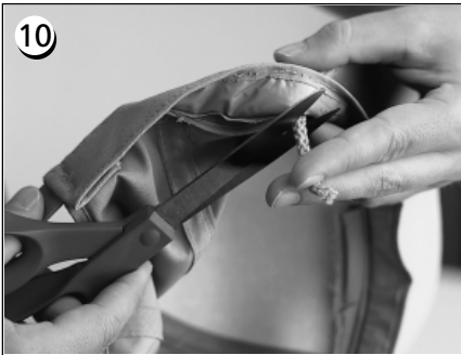
If the braid has a tail on the inside, trim it short to keep it clear of embroidery. Leave only about 1/4" of braid from where it's sewn to the cap.
