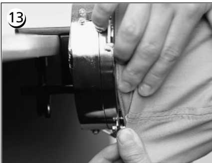
Flatten any "bunching" of the sweatband by folding it over and toward the hoop.
