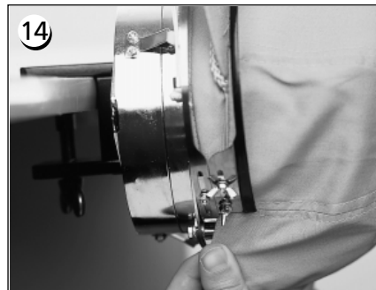
To secure the sweatband, swing the metal strap up and over the sweatband and the cap's brim.
