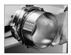
If the posts are bent and touching the cap gauge, bend them back into position.
