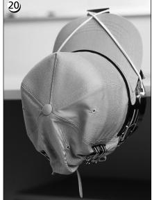
You may now remove the cap hoop from the gauge. Remember to also remove the rubber strip. Your cap is now properly hooped.
