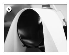
Appropriate backing can now be placed around the rubber strip. The backing stays OUTSIDE the posts and is pushed BENEATH the locator. You may use several layers of backing.
