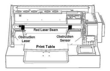
Obstruction Sensor is active only during print operations after PRINT button is pressed. Normally the Obstruction Laser Diode is off. It will first become active as the Print Table
