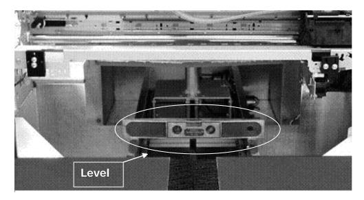
Figure 3.1 Leveling "near" side of printer
