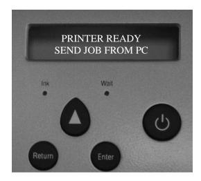
Figure 4.2 Print engine power up complete
