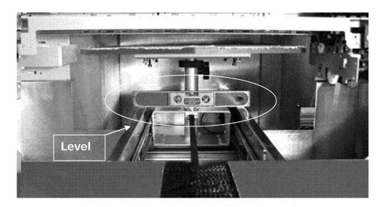
Figure 3.2 Leveling "far" side of printer
