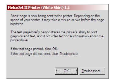
If you receive the above request to print a test page, you will need to lay down a few sheets of standard "8 ½ x 11" white paper on your print table. Be sure to completely cover the table so the Windows test print remains on the paper saving you from cleaning the table.
