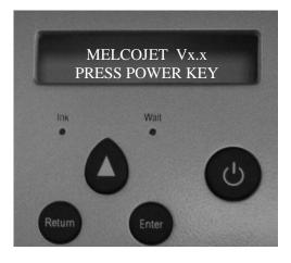
Figure 4.1 Main power on LCD message
