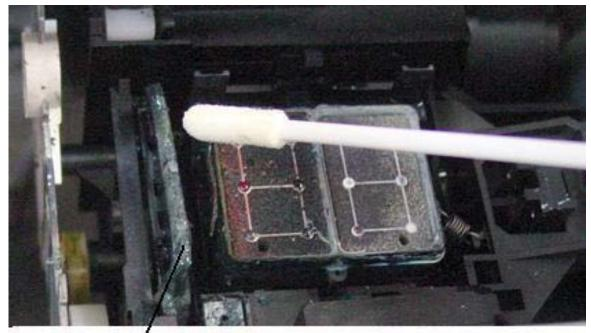
Wiper Blade Cleaning Wiper Blade
