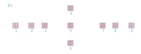
Upon printing the alignment pattern, examine the alignment pattern carefully. For each of the three sets of test patterns, select the square without visible white bands or with the least amount of banding. Consider the example, square number 1 has white vertical bands as does 2,3,4,6,7,8 and 9. However, notice that square number 5 looks mostly whole without any white verticals bands.
