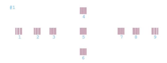
You would enter #5 in the Alignment Adjust window for Section #1. The goal of this test pattern is to produce a print test pattern that has
