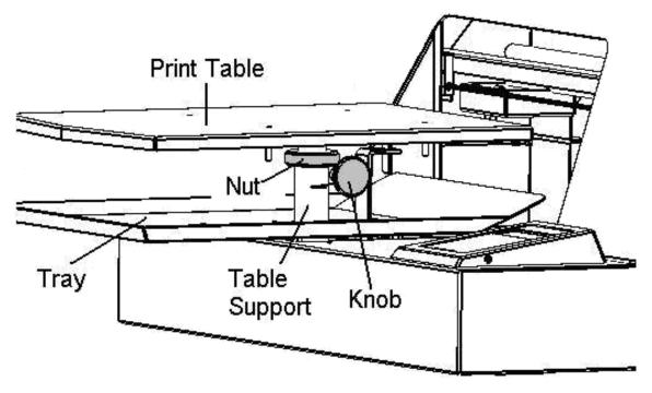
Figure 4.4 Print table adjustment diagram
