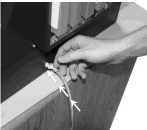
Insert Waste Ink Drain Tube into Waste Ink Drain
