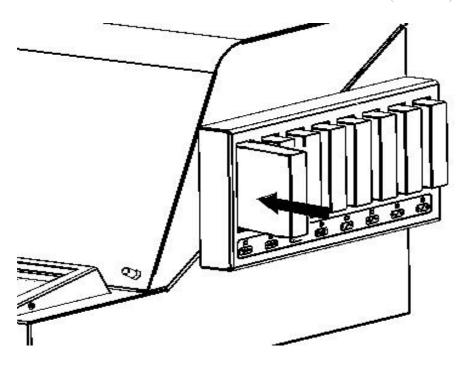
Discard the used cartridges per your local regulations. Never dismantle, tinker with, or attempt to refill the used ink cartridges. Refilled ink cartridges can clog the ink delivery system and printhead.
