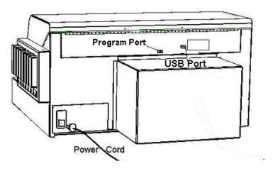
Figure 3.3 plugging in the power cord
