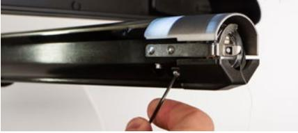
6. Loosen the knobs of the lower shaft support until the top of screws are flush with the t-nut.
