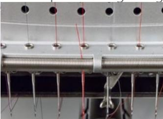
With your hands out of the way, press the adjustment and center keys on the keypad simultaneously to close the grabber and move the thread into the holder behind the needles.
