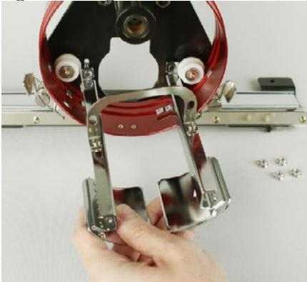
5. Assemble the 4 nuts onto the threaded posts by hand. Allow them to stay slightly loose. This will enable the adjustment of the support wing assembly to the machine.
