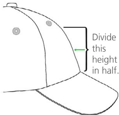
Marking this measurement on the cap with masking tape or tailor's chalk works well. Use the hoop and up or down arrows to move the hoop into position. As you use these keys, the machine's laser will illuminate the placement.
