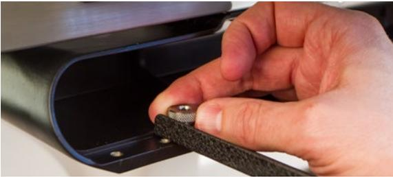
4. Install a hoop by sliding the side brackets of the hoop underneath the spring clips on the support arms. Slide the hoop towards the rear of the machine until it snaps into place and the brackets are fully seated beneath the spring clips. Make sure that the slotted bracket is to the right as you are facing the machine. The support arms will still move a little.
