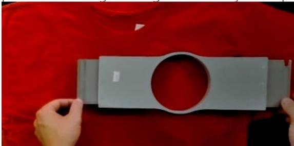
8. Press the hoop down and into place. Take care to press on the ring rather than on the arms. Pressing on the arms can bend the hoop out of shape or break it.
