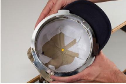
18. The cap is now ready to be placed on the wide angle driver on the machine.
