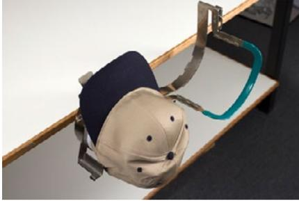
The sweatband may not touch the vertical ridge of the frame. That's okay. Different caps have varying sweatband widths and not all will appear the same when hooped.
