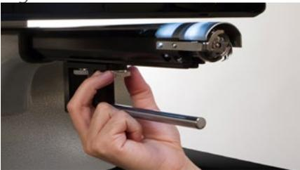
9. Reattach the hook guard by sliding it back into place and tightening the two small screws with a 2mm hex wrench.
