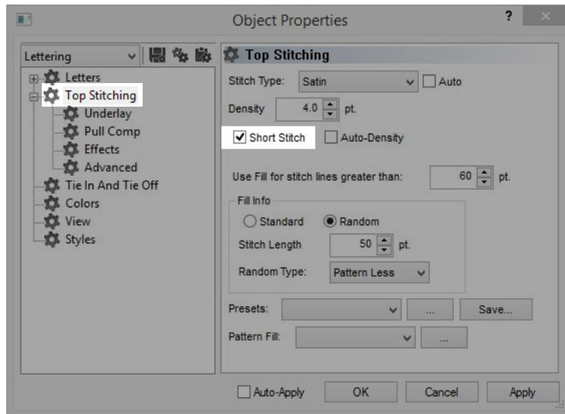
While this feature is beneficial most of the time, it can cause stitches that are too small in smaller lettering or narrow satin stitches. For that reason, since DesignShop V9, a new parameter has been added to the short stitch properties. It will automatically disable for stitch lines shorter than a specified amount. This is set to 20 points by default and should work well for most designs. These parameters can be found under the “Advanced” sub-menu.
