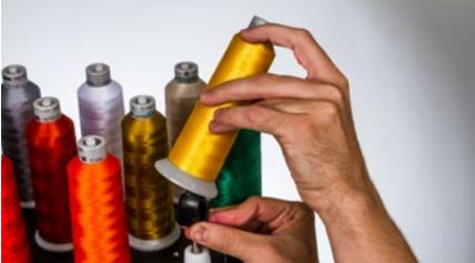
2. If used, black clover may need to be collapsed to allow the new cone onto the thread seat. If the clover is too low on the thread tube, the new cone of thread may not be able to sit securely on the thread seat. If this is the case, move the clover up the thread tube and try again.
