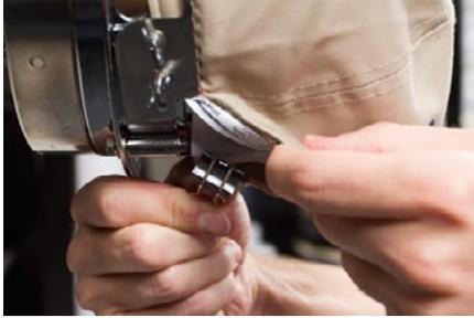
15. If sewing on the sides of the cap, smooth the cap material backward and over the clip posts on the both sides. Indent the cap material along the clip posts.
