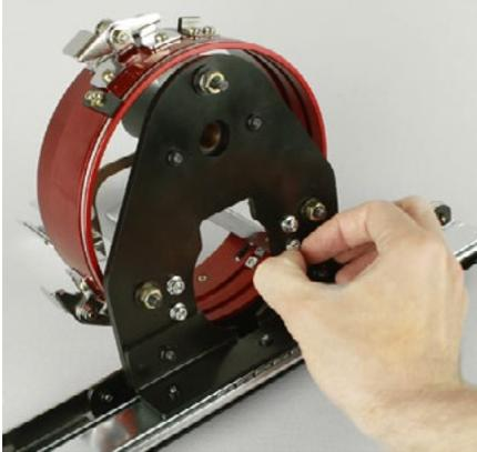
6. With the cap support wing assembly loosely installed on the wide angle driver, install the driver onto the machine.
