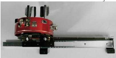
6. Move the driver back and forth a few times to spread the grease.
