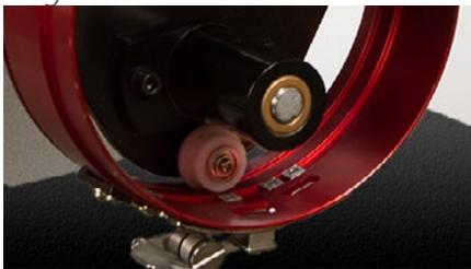
3. Place a business card of medium to heavy stock (or equivalent) between the needle plate and the driver ring. A single business card should be able to slide between them with little resistance. A gap of two business cards is acceptable.
