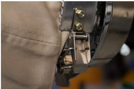
12. The cap frame strap may need to be tightened if it does not fit the cap snugly or loosened should it be too tight to fasten appropriately. This is only necessary when hooping a different style of cap for the first time using the cap frame. Subsequent hoopings of that style should fit well after the adjustment.
