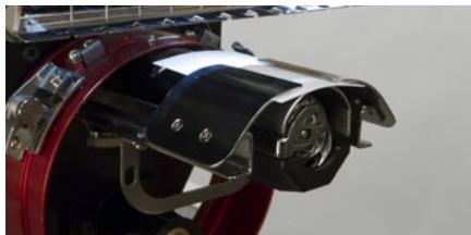
10. Adjust one side of the cap support until it makes contact with the business card and needle plate. Tighten the two nuts on the back of the driver.
