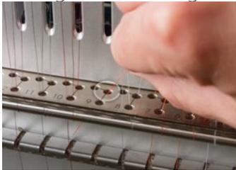
6. Bring the thread around the thread sensor from back to front and up through the front hole of the middle thread guide.
