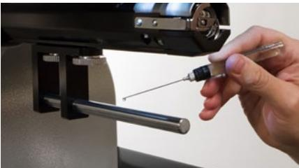
11. Slide the red driver assembly onto the lower arm and support shaft. This may be easier if the grabber bar of the machine is closed. To close the bar, simultaneously press the "Adjustment" and "Center" keys on the keypad of the machine.
