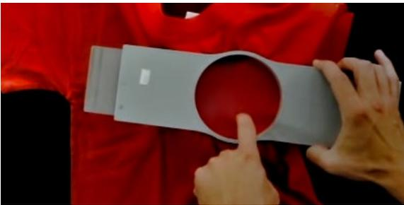
10. Check the back of the hooped piece. Make sure that there are not wrinkles or other parts of the garment lodged in the hoop.
