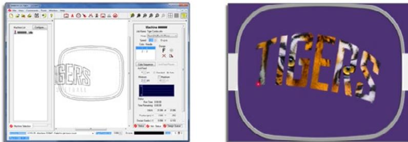
Now that the first point has been entered, use the hoop and the arrow keys on the machine keypad to move the hoop on the machine so that the laser light is on the second reference point on the garment. In the example, the vector line was digitized with the left input point first. This is the first reference point.
