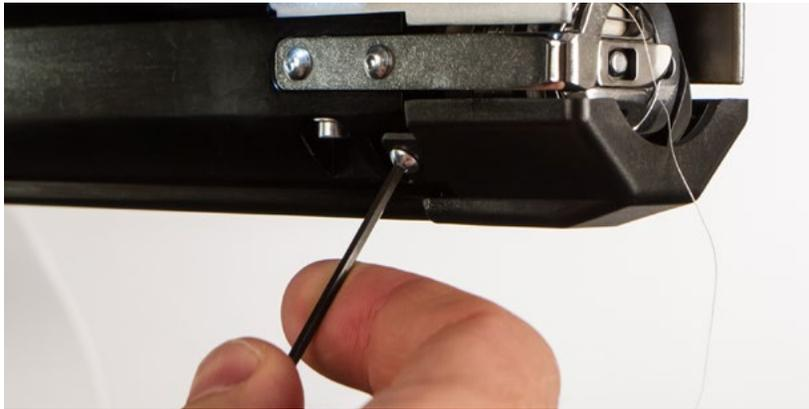
3. Remove the needle plate by removing the two allen screws that secure it.
