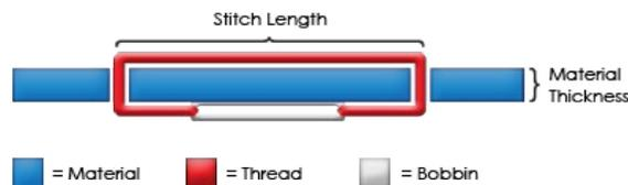
In general, as material to be embroidered increases in thickness, the value for the material thickness should be higher to increase thread feed.
