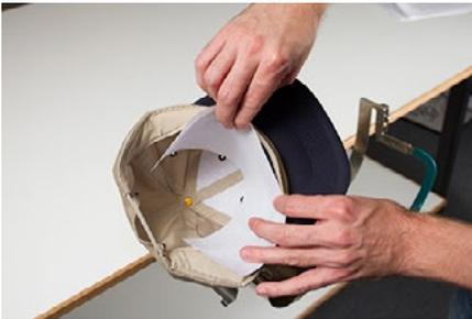
4. Slide the prepared cap onto the cap frame with the visor pointing up and the frame going inside the cap. Make sure that the sweatband is flipped to the outside of the cap.
