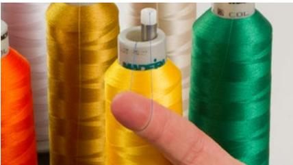
6. Tie the end of the old thread to the end of new thread using a square knot.
