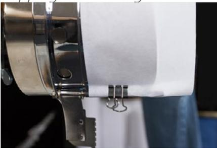
4. Slide the prepared cap onto the cap frame with the visor pointing up and the frame going inside the cap. The bill should be pushed against the bill-stop on the frame. The bill should also be
