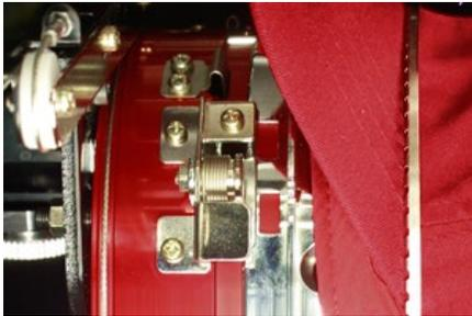
3. Rotate the hooped cap 90° so the bill can pass under the needle case. The hoop can now be removed from the machine.
