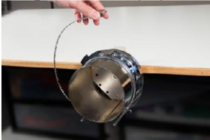
3. Place an appropriate backing over the gauge and the teeth of the cap frame. Make sure that the backing is long enough to support the full embroidery area. It may be easiest to use backing long enough to reach the posts on the bottom of the cap frame.
