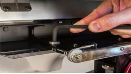
2. Slide the red driver assembly toward you and off of the lower arm and support shaft. This may be easier if the grabber bar of the machine is closed. To close the bar, simultaneously press the "Adjustment" and "Center" keys on the keypad of the machine.
