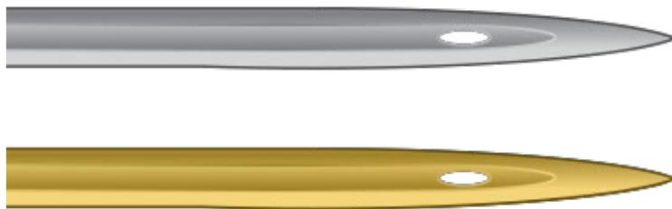
Titanium needles are gold in color and offer an extended sewing life of 2 to 3 times the life of a standard needle. While they are stronger needles, they have little flex. If deflected, they will often break instead of bend. Titanium needles are usually marked with a “PD” on the packaging.
