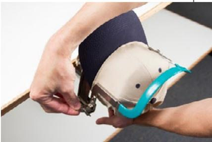
10. While holding the cap frame strap down around the sweat band, release the back of the cap and attach the strap latch over the hook on the support. Pull the tab to latch the cap frame.
