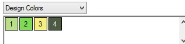
3. In the example above, the first recommended color is a light green. The second color is medium green. If you wanted to sew in those colors, find the light and medium green threads on the thread tree of your machine. The position of the cones of thread on the machine correlates to the positions on thread cone display in the software.
