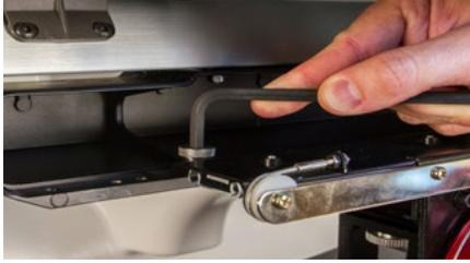
2. Slide the red driver assembly toward you and off of the lower arm and support shaft. This may be easier if the grabber bar of the machine is closed. To close the bar, simultaneously press the "Adjustment" and "Center" keys on the keypad of the machine.
