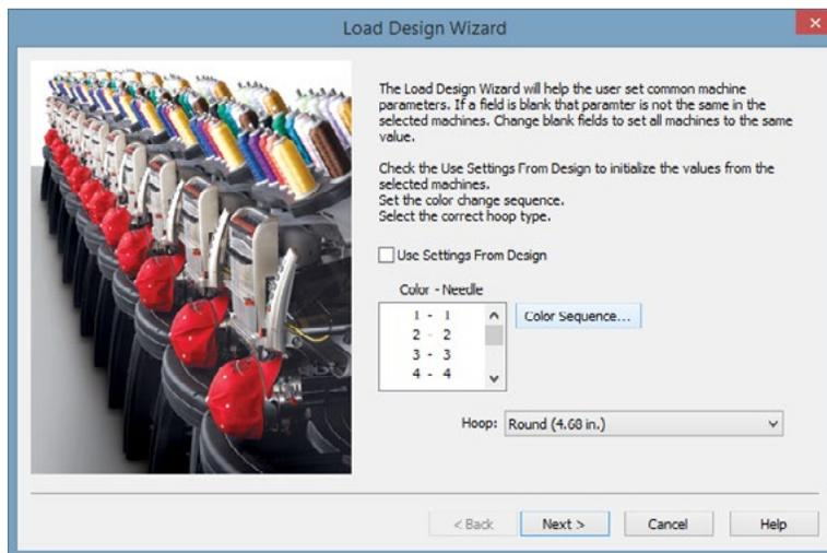
4. After a loading progress bar displays, the design will appear on screen and be loaded into your machine. The next window of the wizard will appear, and you can set the color sequence.
