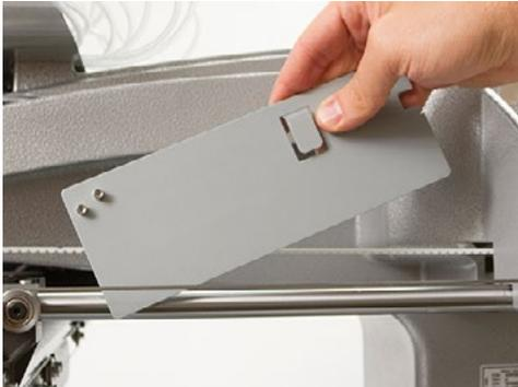
A close-up photograph showing a person's hand lifting a grey rectangular x-cable tension gauge away from the machine's frame. The gauge has a small metal tab and two screws.                                                                                                                                                | <p>"Remove Gauge<br/>Remove the x-cable tension gauge before proceeding.<br/>Press the next button to continue."</p>
