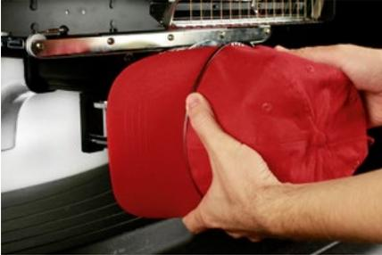
2. Rotate the bill back up so that it is behind the needle case and the location tab on the driver aligns with the notch in the frame.
