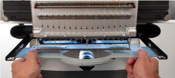
5. Using the installed hoop as a guide, square up the support arms.
