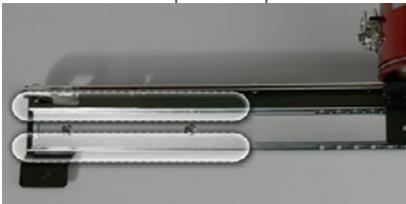
4. Apply a thin film of hp grease to the grooves of the slider bearing.
