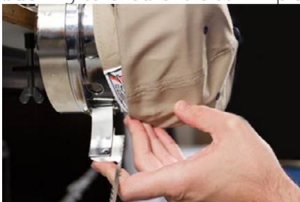
8. When the left side of the cap is within the strap hinge post, swing the strap up and over the cap brim. On the side of the cap, the teeth of the strap should fall just above the seam attaching the
