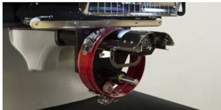
8. Move the driver and carriage back until the cap support wing assembly fully covers the needle plate.
