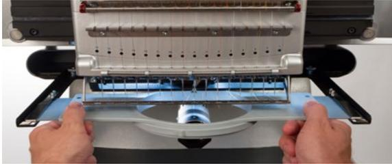
2. Slide the hoop towards the rear of the machine until it snaps into place and the brackets are fully seated beneath the spring clips.
