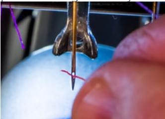
11. Be sure to align the thread with the small v-notch in the thread feed cover.
