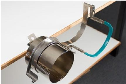
3. Place an appropriate backing over the gauge and the teeth of the cap frame. Make sure that the backing is long enough to support the full embroidery area. It may be easiest to use backing long enough to reach the teeth on each side of the cap frame.
