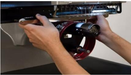
3. Remove the hook guard by loosening the screws on both sides of the lower arm using a 2mm hex wrench, and sliding the hook guard forward. The screws do not need to be completely removed.
