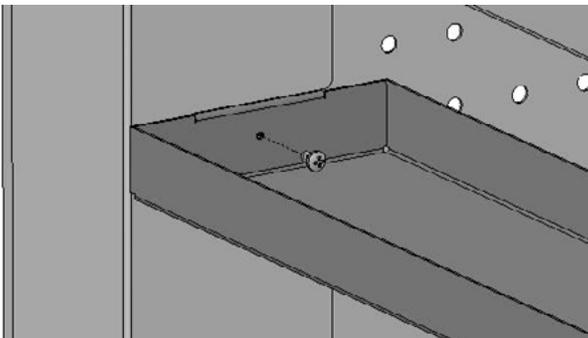
Align the holes in the tray and the cart legs. Tighten it into place using the two sheet metal screws (Items 2).
