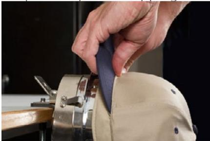
7. Pull the side of the sweatband toward the cap frame and down. Smooth any bunching of the cap sides or sweatband. You may eventually need to fold the sweatband a bit to avoid the latching hook. But this will help with the placement of the cap on the frame. As you do this, watch the backing to ensure it is still in place.
