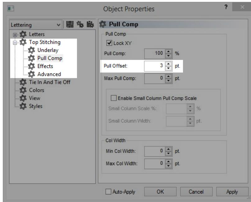
Pull offset extends the stitch lines of an element by adding the specified amount to each side. If the element was 5 points wide at the thinnest point, a "3" could be entered into the pull offset field to extend the stitch lines by three points on each end. This would create an element that at the thinnest point is now 11 points wide and thick enough to sew without breaking a thread.
