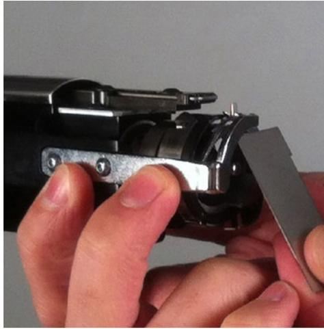
3. Holding the hook support from the side with the adjustment screws, adjust the position of the hook support to the requirements from the inspection procedure above.
