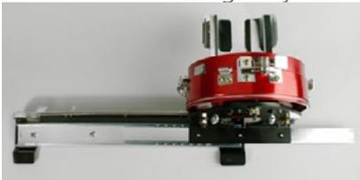
3. Clean the exposed portion of the exposed slider bearing groove with a clean towel.
