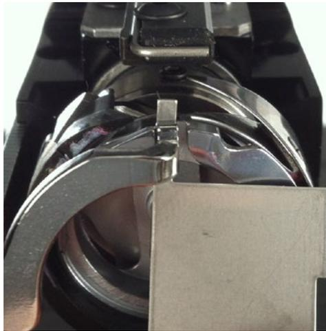
5. Tighten the two screws holding the hook support.
