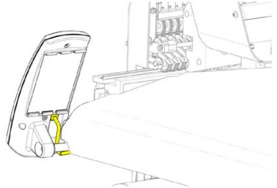
Route the network cable (shown in yellow) from under the right side machine cover, under the user interface mounting bolt, and plug into the back of the user interface assembly.
