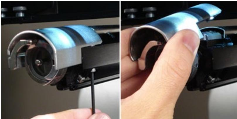
4. Using compressed air or a brush, remove any thread or lint buildup from the area.
