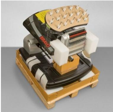
4. Cut the packing/holding straps securing the machine to the box/pallet. Remove any additional loose packaging, boxes, and foam spacers.
