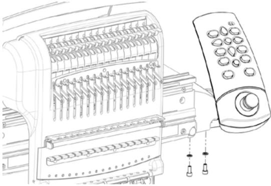
Using the two screws and two lock washers that came with the user interface assembly, attach the interface as shown in the image using a 4mm hex wrench.
