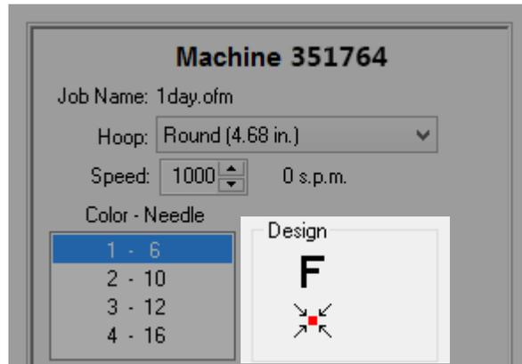
Every click on the orientation F will rotate the icon by 90°. When the clicking stops, the design will rotate and the F icon will reset. The icon does not show the orientation of the design. It shows the changes you are making.
