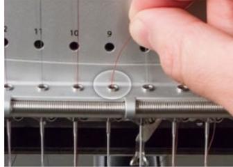
10. Thread the needle from front to back. Cutting the end of the thread may allow it to more easily pass through the eye.
