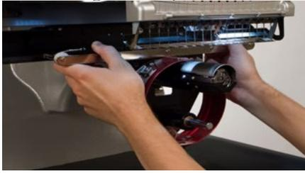
12. Using two of the thumb screws from the hoop arms, attach the red driver to the x-carriage of the machine. The driver will attach to the two innermost holes. Tighten them to finger-tight, and then use a 6mm Allen wrench to tighten an eighth to quarter turn more. Do not over-tighten the screws as they are designed to break before damage to the machine can occur.
