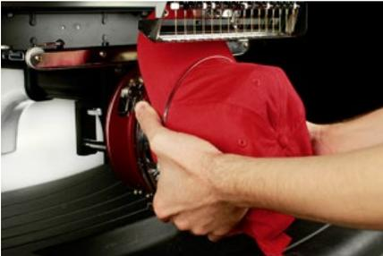
3. This also aligns the rectangular holes along the edge of the frame with the spring loaded locking clamps on the driver.
