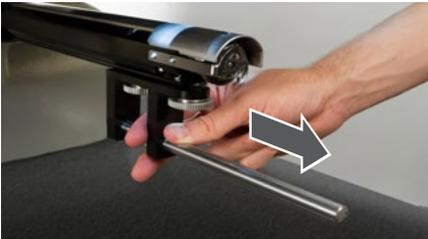
5. Reattach the hook guard by sliding it back into place and tightening the two screws using a 2mm hex wrench.
