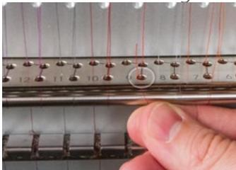
7. Pull the thread up and through the eye of the take-up lever from right to left.
