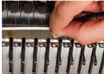
5. Pull the thread down to the middle thread guide. Of the three holes, push the thread from the top through the back right hole. Make sure the thread is on the right side of the take-up lever.
