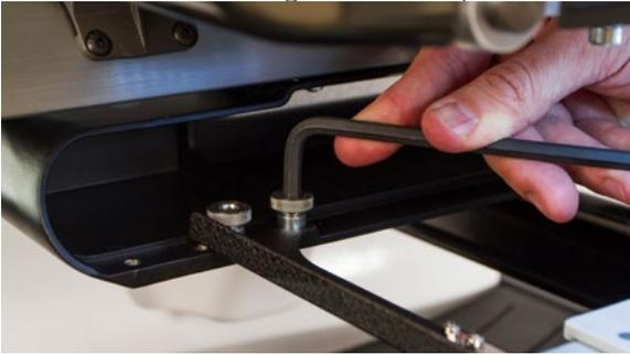
*If the hoop brackets shift forward and back, the spring clip may need to be adjusted. See the information below.*
