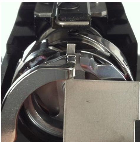
The retaining finger gauge should slide between the hook support and the hook basket with no resistance. The gap between the hook support and the hook basket should be no more than 1.1 times the thickness of the gauge. (The gauge is 0.020', and the tolerance is +/- 0.002')
