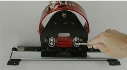
4. Remove the cap support wing assembly. Slightly pivot the assembly from left to right and back again while removing it. This will help to ease each leg around the roller.
