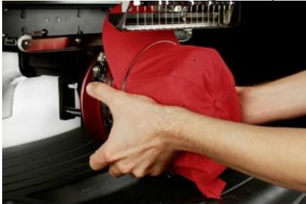
2. This will allow the frame to release and be pulled free from the driver.
