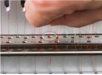
9. Press the thread into the felt restraint and feed it down through the lower thread guide.
