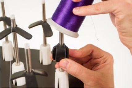
3. Releasing the clover will cause it to expand inside the cone core and stabilize the thread cone.
