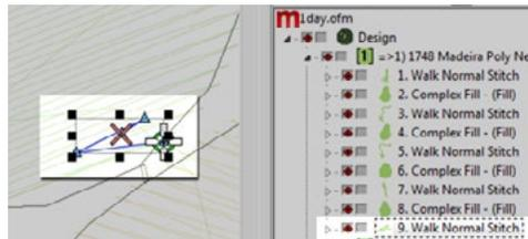
In expanded stitch files, these tie stitches are a bit harder to see because you cannot just select the last element before a trim.
