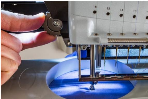
6. Turn the gear with your fingers to adjust the presser foot height up or down as needed.
