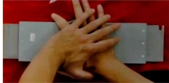
9. Once the material has been hooped, make sure that the garment is smooth, flat, and taut. If the garment is loose, you may need to remove the hoop and adjust the hoop tension or hooping method.
