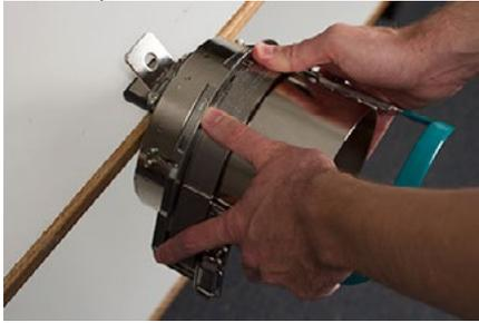
2. Unlatch the cap frame and swing the frame open and to the right. Do this by pulling the tab away from the frame. Then, press down on the edge of the frame to free the latch from the hook. Swing the frame open.
