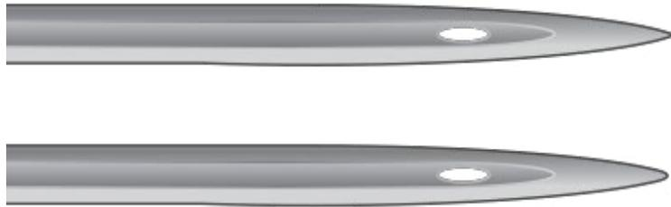
Ball point needles are most often used on knit materials. They tend to move the threads of the material to the side of the needle as they sew. Ball point needles are usually marked with a “BP” on the package.
