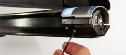
4. Loosen the knobs of the lower shaft support. Then, slide the lower support shaft out of the t-channel and off the machine.
