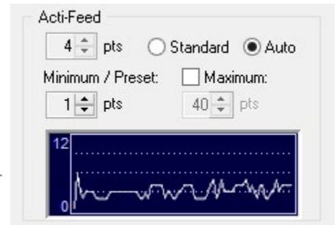
**i** *While auto mode was designed for materials that change thickness, it works well with most materials. It is recommended for your first sew-outs.*
