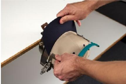
8. Gently pull from the back of the cap. This will pull the cap down and snug against the frame.
