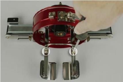
3. Remove the four nuts on the back of the driver. A 7mm hex driver or wrench will be needed.
