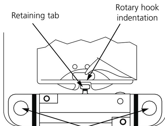
Holes for screws which mount from below
