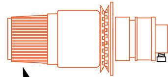
Rotate to adjust tension
