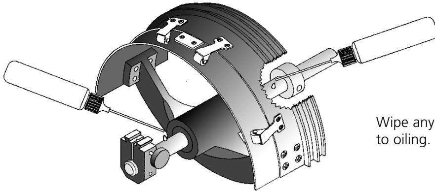
Wipe any lint off the shaft prior to oiling.
