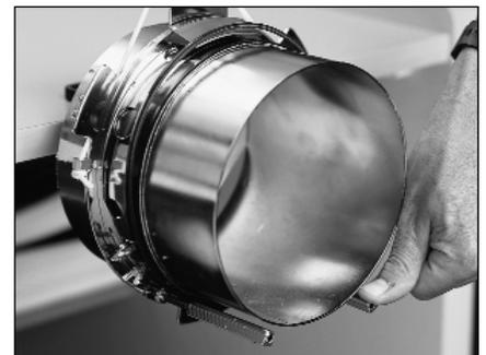
If the posts are bent and touching the cap gauge, bend them back into position.
