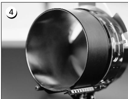
For the best sew quality, use the rubber strip; it provides appropriate spacing and hoop tension. Drape the strip over the gauge...
