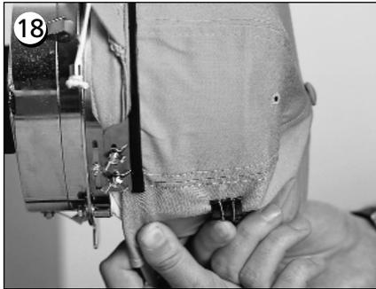
Pull the elastic brim holders over the cap's brim to the front. Pull the wrinkles out of the cap using light tension. To secure the cap fabric, attach two clips...
