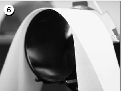
Appropriate backing can now be placed around the rubber strip. The backing stays **OUTSIDE** the posts and is pushed **BENEATH** the locator. You may use several layers of backing.
