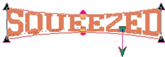
**Diamond** - Click the left mouse button on the line above the text (this will insert a triangle control point). Click the left mouse button on the line below the text (this will insert a triangle control point). Hold down the (Ctrl) key and left click the other triangle control point. Hold down the (Shift) key, click on one of these control points and drag it away from the center of the text.
