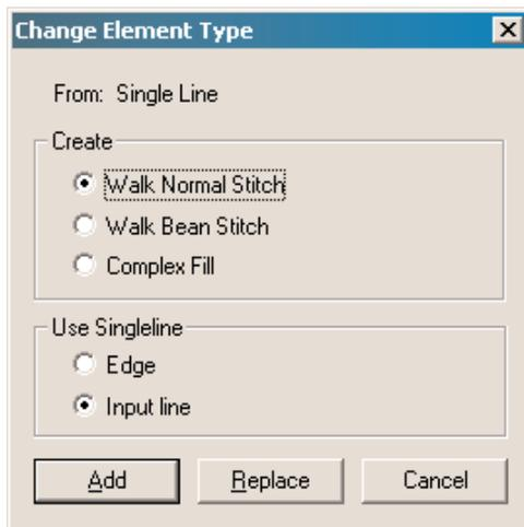
In the case of the Singleline Column, you also have the option to use the edge of the column or the input line. When using the "Edge" complex fill is no longer an option but singleline is added to the list. Using the "Edge" is used when wanting to put a border around a singleline column.
