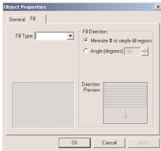
The Fill page is displayed allowing settings that are applicable to fill stitch objects to be modified.
