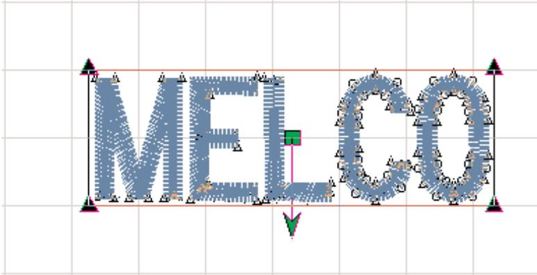
To rotate the element: you will use the green arrow that comes from the middle of the element. You can click and drag the center green box to have the center of rotation anywhere that you would like. Once you have determined the center of rotation, click and drag the green arrow in the direction that you would like your element to rotate.
