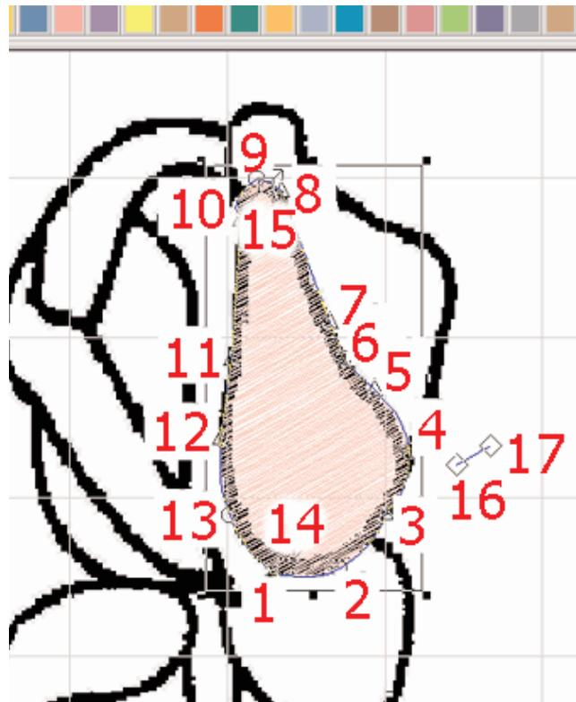
After inputting the last point of the complex fill, press the Enter key.
