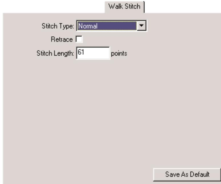
**Retrace:** When you digitize a walk stitch and have the retrace on, the walk stitch will be stitched out twice, the second walk stitch on top of the first walk stitch. This is useful in making a single walk stitch appear thicker. To turn this function on, left click in the box next to "Retrace." A check mark will appear to symbolize that this function is on. Click again to remove the check mark, which symbolizes that this function is off.
