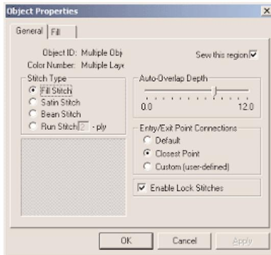
The Object Properties Dialog Box. Shown above are both pages (i.e. tabs) of the object properties dialog box. The General page is displayed allowing settings that are applicable to all types of objects to be modified.
