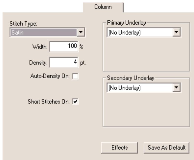
8. Click the down arrow at Primary Underlay and choose an underlay (choose a secondary underlay if necessary).
