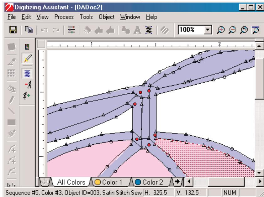
The light blue color of the FunHat object indicates that it will be generated using satin stitches. Larger red circles at the centers of column intersections indicate control points that may be clicked upon to provide alternatives to a chosen intersection's interpretation. Also, displayed are the detected outlines of the objects. A segment containing a circle indicates a detection of the smooth arc (curved input point), while small squares indicate straight line segments (straight input points).
