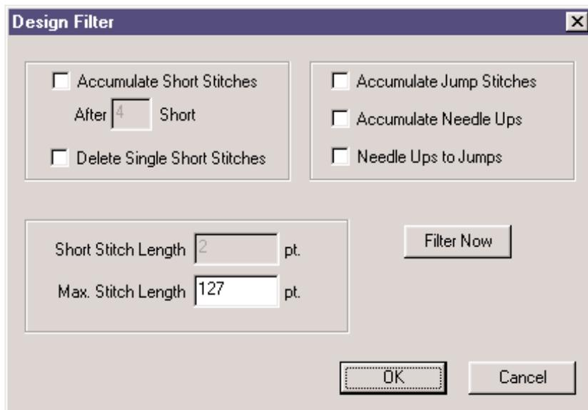
Turn on the functions that you wish to affect your design by left clicking in the box next to the function (click again and the check mark, that was just inserted, will be removed). A check mark in the box symbolizes the function is ON, whereas no check mark in the box symbolizes that the function is OFF.
