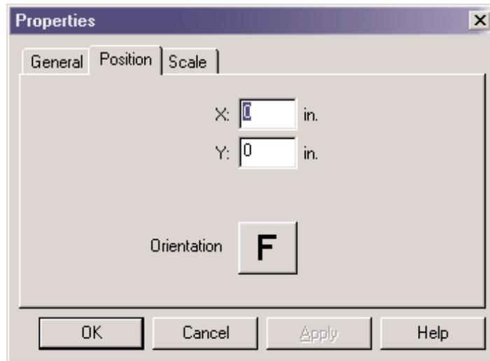
Position represents the number of embroidery points (1/254th of an inch) that the center of the image is offset from the center of the design (or View Window). This allows you to move your image with respect to the design.
