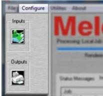
The “Inputs” and “Outputs” buttons launch the MelcoRIP configuration dialogs for inputs (Hot Folders, Printer Entities, etc.) and outputs (Output Queues) respectively. These options are also present under the “Configure” menu option. These are described in more detail in the [Manage Inputs](#) and [Manage Outputs](#) sections.
