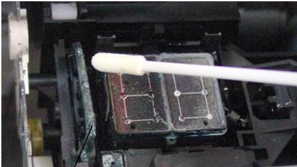
**Wiper Blade      Cleaning Wiper Blade**
