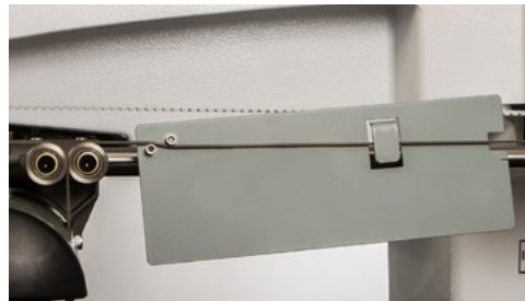
Figure 5: Positioning the X-Cable Tension Gauge
