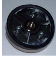
Figure 3 - Screws On Back of Take-Up Lever Cam
