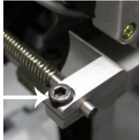
Figure 3 - Loosen Top Screw
