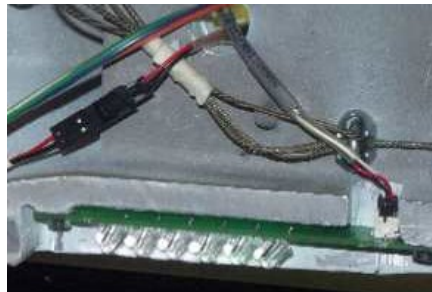
Figure 6 - Right LED Cluster Harness
