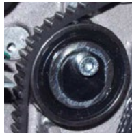
Figure 3 - Z-Belt Idler Pulley
