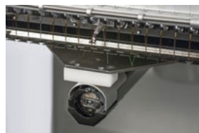
Figure 2 - X/Y-Home Fixture in Needle Plate Hole
