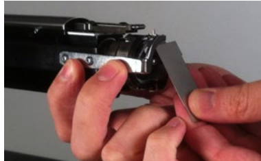
Figure 3 – Hook Support Adjustment
