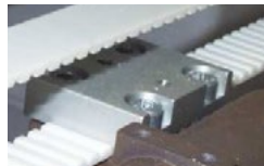
Figure 3 - Right Y-Drive Timing Belt Clamp
