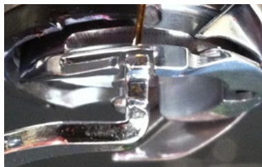
Figure 2 – Rotary Hook Basket Notch
