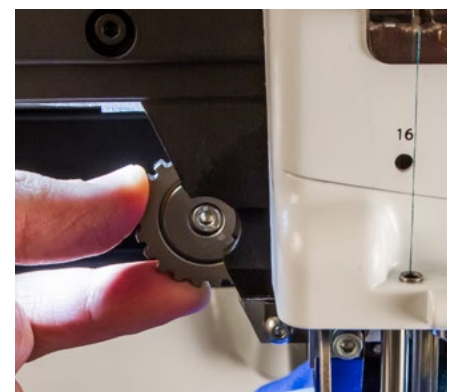
Figure 2 - Presser Foot Height Adjustment Eccentric
