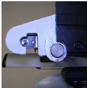
Figure 10 - Cable Tensioning Bracket (Left side of machine)
