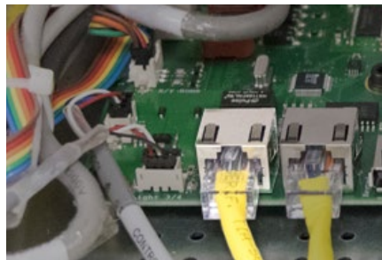
Figure 3 - Ethernet Connector Location on Main PCB ("Eth")
