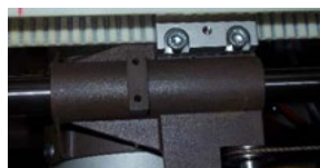
Figure 1 - Bearing Block Assemblies
