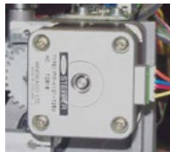
Figure 1 - Thread Feeder Stepper Motor
