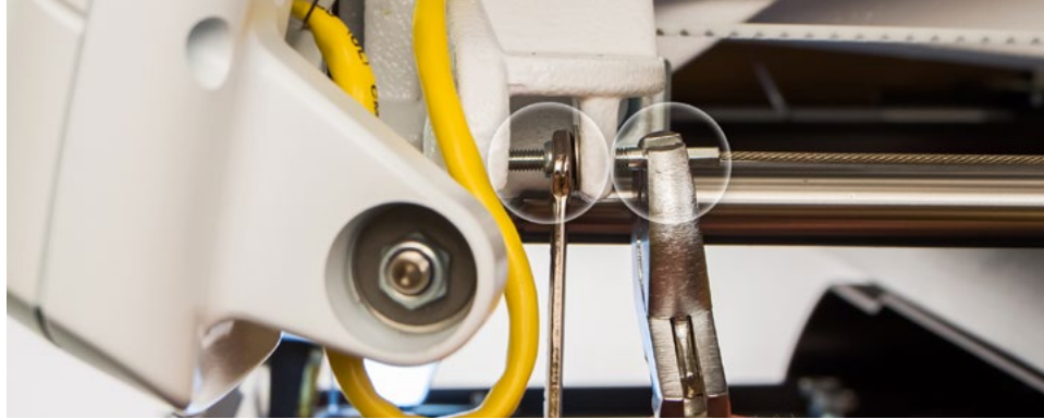
Figure 7:X-Cable Tension Adjustment
