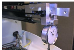
Figure 4 - Dial Indicator Installed on Needle Plate Bracket
