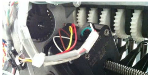
Figure 1 - Color Change Harness Connection to Motor
