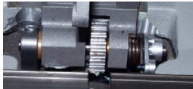
Figure 2 - Take-Up Lever Drive Gear Assembly
