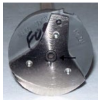
Figure 2 - Remove Center Screw
