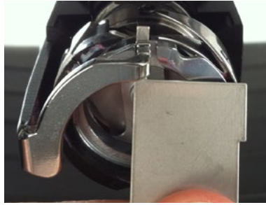
Figure 5 – Retaining Finger Gauge Usage
