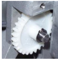
Figure 1 - Thread Feeder Gear
