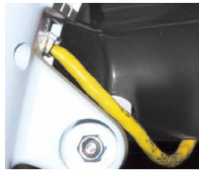
Figure 2 - Keyboard Harness Connection
