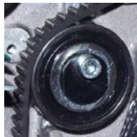
Figure 1 - Z-Belt Idler Pulley
