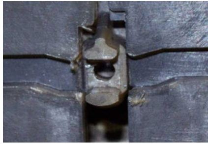
Figure 1 - Reciprocator Drive Groove at "Head Up" Position
