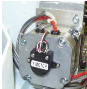
Figure 3 - Harnessing Routed Under Y-Motor
