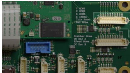
Figure 4 - Grabber/Thread Feed Motor Connection at PCB
