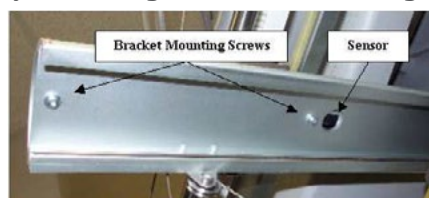
Figure 2 - X-Home Sensor and Mounting Screws
