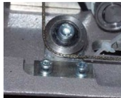
Figure 8 - Left Rear Cable Pulley
