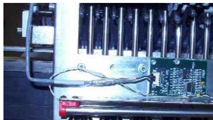
Figure 1 - Threadbreak Harness Connected to Sensor PCB
