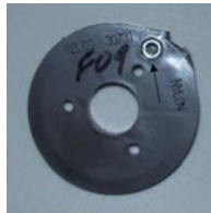
Figure 4 - Remove Hex Nut
