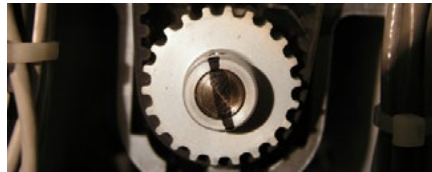
Figure 3 - Lower Z-Shaft Drive Pulley
