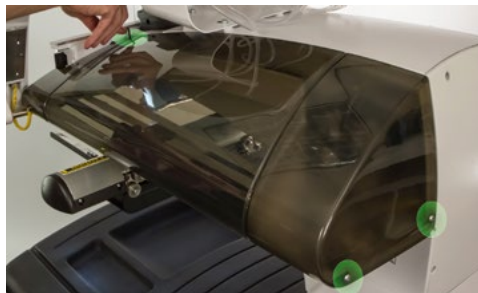
Figure 2: Removing the right cover
