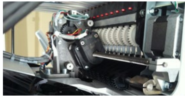
Figure 1 - Color Change Linear Actuator
