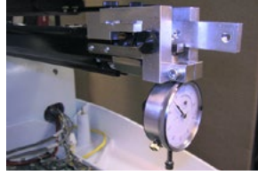
Figure 3 - Dial Indicator and Adaptor Installed on Lower Arm Extrusion
