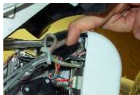
Figure 2 - Thread Feed Motor Lead
