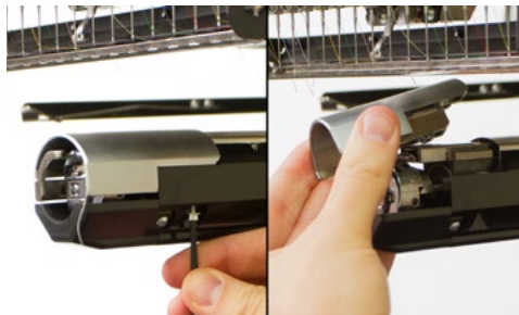
Figure 2 – Needle Plate Screws
