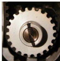
Figure 2 - Lower Z-Shaft Pulley
