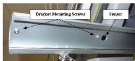
Figure 2 - X-Home Sensor and Mounting Screws
