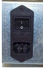
Figure 1 - Power Input Switch (with fuse)
