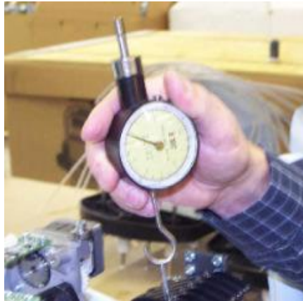
Figure 1: Measurement of Take-Up Lever Pull Force
