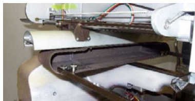
Figure 1 - X-Beam and Carriage Installed on Machine
