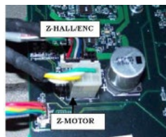
Figure 2 - Z-Motor PCB Connections
