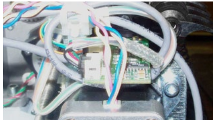
Figure 4 - Grabber/Thread Feed Motor Connection at PCB
