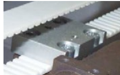
Figure 3 - Right Y-Drive Timing Belt Clamp
