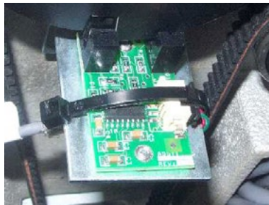
Figure 1 - Connection to Z-Index PCB
