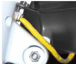
Figure 1 - User Interface Harness Connection
