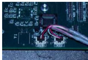
Figure 5 - LED Cluster Harnesses Connected at Main PCB
