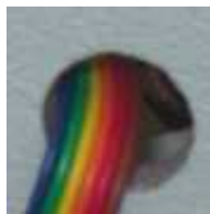
Figure 3 - X/Y Home Harness Access Hole
