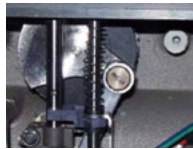
Figure 1 - Take-Up Lever Connecting Arm
