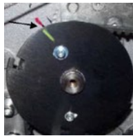
Figure 2 - Index Mark on Z-Index Flag
