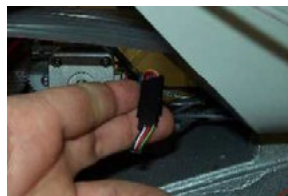
Figure 1 - Grabber Motor Lead
