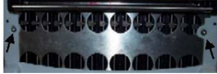
Figure 2 - Needlecase Access Cover Removed
