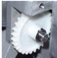
Figure 1 - Thread Feeder Gear
