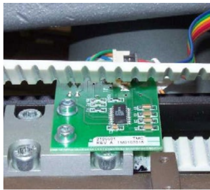
Figure 1 - X/Y Home PCB (Belt turned up for illustration)
