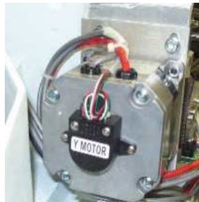
Figure 3 - Harnessing Routed Under Y-Motor
