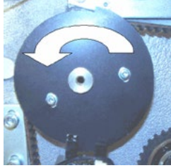
Figure 3 - Turn Z-Axis Flag Counter-Clockwise (CCW)
