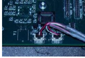
Figure 5 - LED Cluster Harnesses Connected at Main PCB
