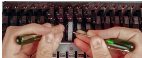
Figure 2 - Prying Thread Feeder Roller Loose
