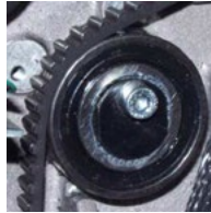
Figure 3 - Z-Belt Idler Pulley
