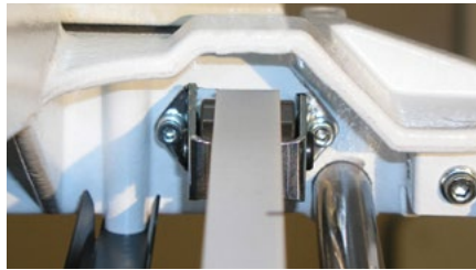
Figure 3 - Y-Drive Timing Belt Adjusting Screws
