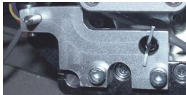
Figure 4 - Left Color Change Spindle Mounting Bracket
