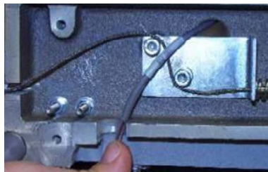
Figure 1 - Left LED Cluster Harness
