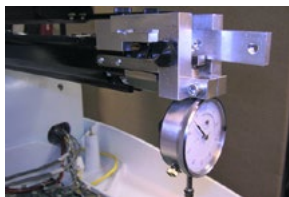
Figure 4 - Dial Indicator Installed on Needle Plate Bracket
