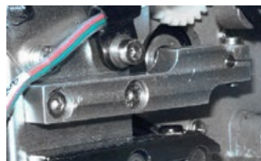
Figure 2 - Right Color Change Spindle Mounting Bracket
