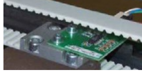
Figure 2 - Left Timing Belt Clamp and X/Y Home PCB
