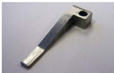
Figure 1 - Z-Home Sensor Fixture
