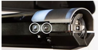
Figure 1 – Hook Support Screws
