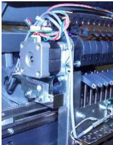
Figure 4 - Routing of Harness to Top of Needlecase
