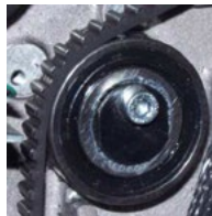
Figure 1 - Z-Belt Idler Pulley
