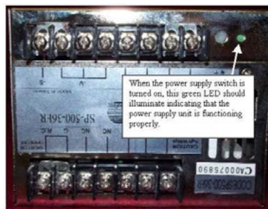
Figure 3 - Power Supply Indicator LED
