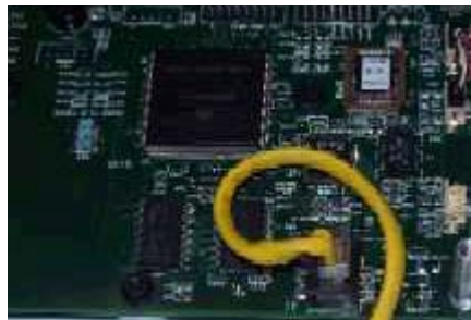
Figure 3 - Ethernet Connector Location on Main PCB (J1)
