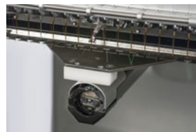
Figure 2 - X/Y-Home Fixture in Needle Plate Hole
