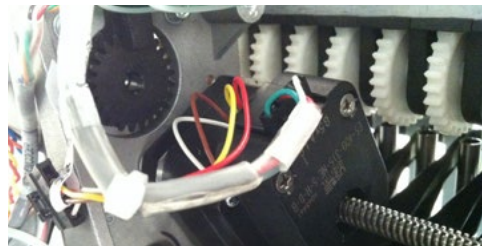
Figure 1 - Color Change Harness Connection to Motor
