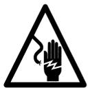
Shock hazard. No user replaceable parts behind this label. Do not open!
