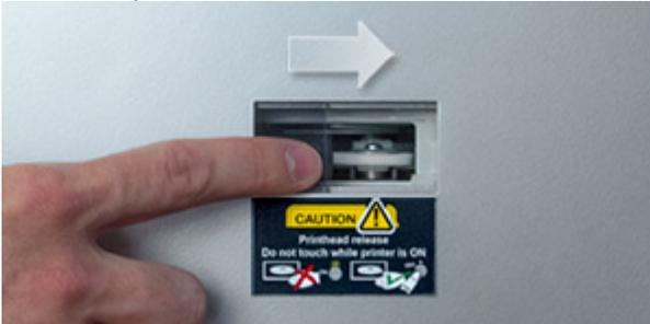
***Do not leave the print head off of the capping station longer than 15 minutes. There is a danger if that time should be exceeded that the print head may dry out.***
