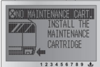
7. Insert the maintenance tank into the printer and close the maintenance tank cover.
