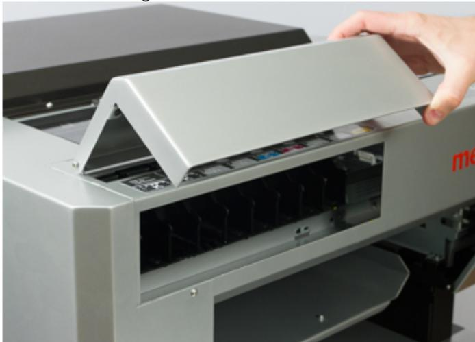
2. Slide each cartridge into the appropriate bay as shown above. Slide into place until you hear a click.
