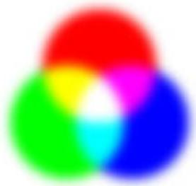
The additive color system works with projected light. Computer monitors and televisions use this model. Light comes from the screen and is viewed by people directly with nothing reflecting the light.
