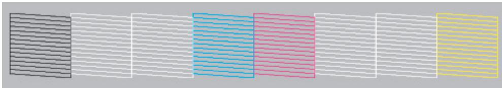
Make sure that the ink assignment is correct and as shown. If you see any gaps as shown below, perform a power cleaning from the printer control panel.
