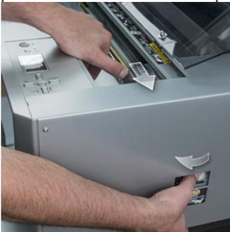
10. Close the printer cover and slide the maintenance cover closed.
