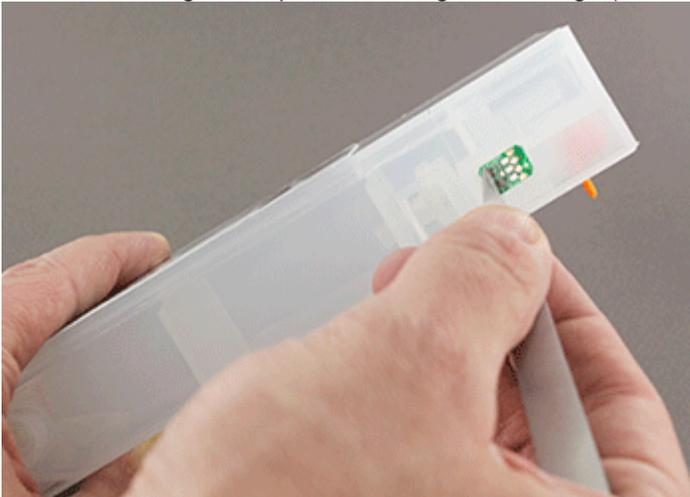
3. Install the original Epson chip in its dedicated place on the refillable cartridge.
