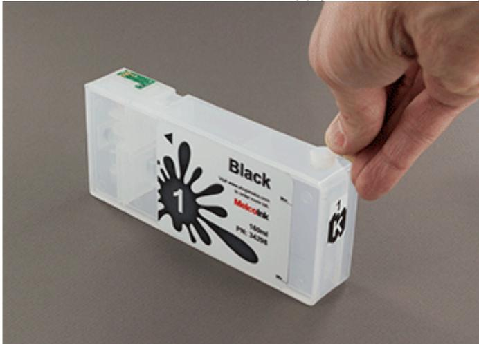
2. Use the funnel provided with the printer to fill the cartridge with its respective ink. It is advised that the ink level does not exceed 90% of the maximum capacity marked on the label.
