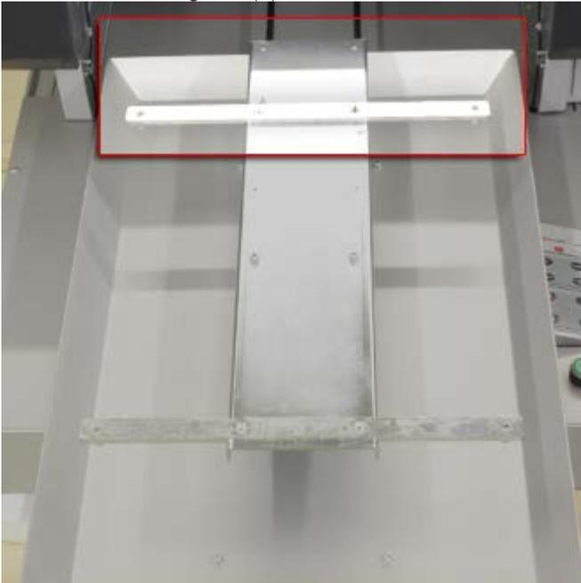
5. Align the Polo Table as shown in the picture below and secure it to the Table Support using four (4) M4 Countersunk Hex Screws.
