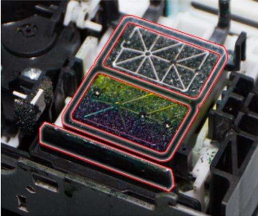
9. After cleaning the capping station and wiper, use a syringe or dropper to fill the capping station with clean cleaning fluid. This will prevent the print head from drying out over a longer period.
