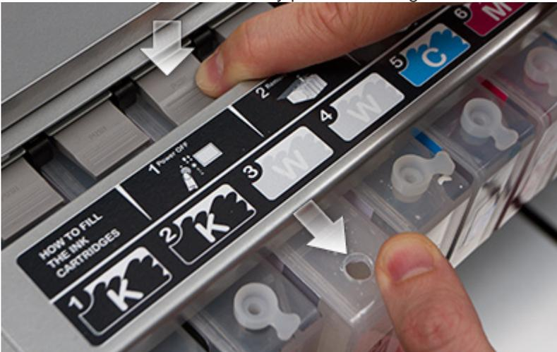
4. Replace the rubber seal to prevent the spillage of ink.
