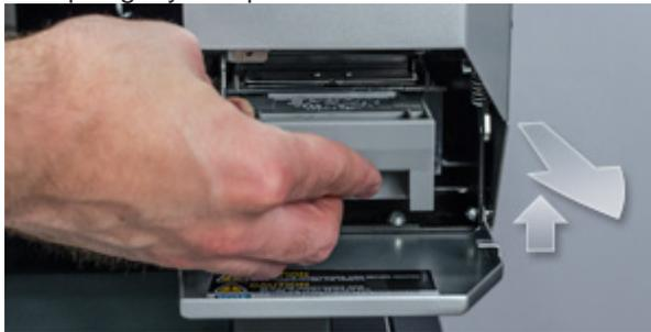
2. Empty and properly dispose of the remaining ink from the maintenance tank. Make sure to not get ink on the maintenance tank chip.
