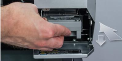
8. While the maintenance tank is NOT installed, eject the table by pressing the eject button on the table control panel.
