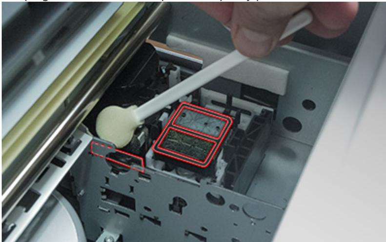
6. After cleaning the capping station and wiper, use a syringe or dropper to fill the capping station with clean cleaning fluid.
