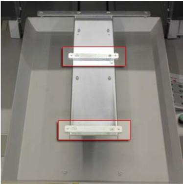
4. Align the Small T-Shirt Table and the Adapter Plate as shown in the picture below and secure them to the Table Support using six (6) M4 Countersunk Hex Screws.
