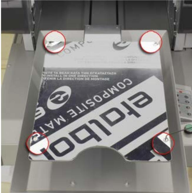
*When shipped, the tables may be covered in a protective film. This film should be removed before use. Most of the images in this section show the tables with the protective film.*
