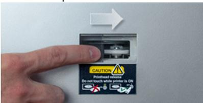
***Do not leave the print head off of the capping station longer than 15 minutes. There is a danger if that time should be exceeded that the print head may dry out.***
