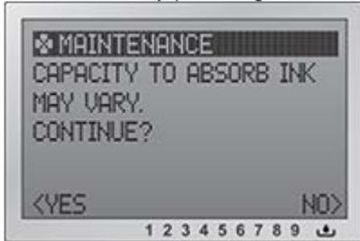
***If the ink level icon of the maintenance tank remains blank ("NON-GENUINE") the user must always check visually the real ink level of the tank and empty it when needed.***
