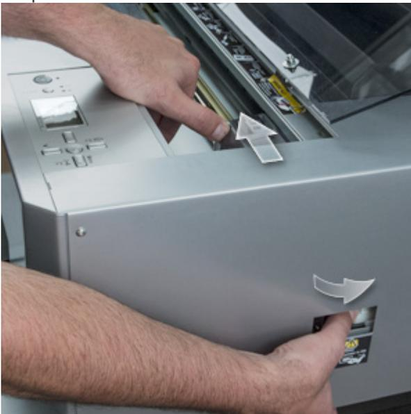
6. Move the print head by hand to the far left side of the printer. This will allow you free access to the capping station and the wiper.
