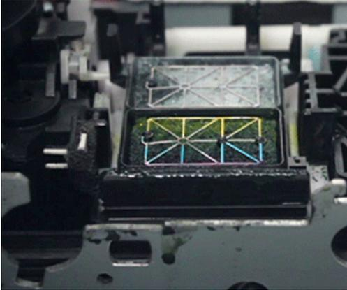
8. Carefully clean around the capping station and the wiper blade with a cleaning applicator dipped in the cleaning solution from the small container in step 2 above. Make sure that the rubber parts of both the wiper and the capping station are always clean and free from any ink, dried ink, dust, or dirt. These two are the only parts of the printer that contact the print head. Keeping these clean will help ensure quality prints.
