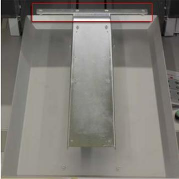
3. Mount the two (2) Short Table Interface Brackets in the locations shown below using M4 Countersunk Hex Screws.
