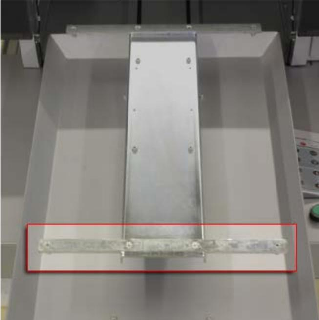
4. Mount the Rear Long Table Interface Bracket you removed in step 2 above in the location shown below using two (2) M4 Countersunk Hex Screws.
