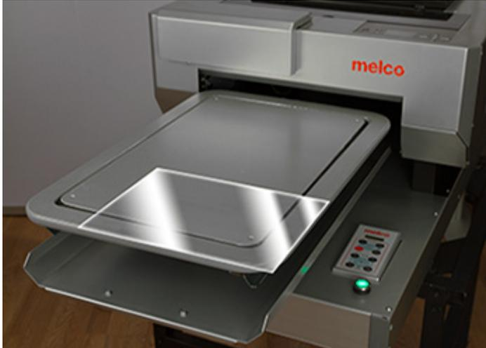
3. Adjust the height of the table by pressing the Auto button on the table control panel.
