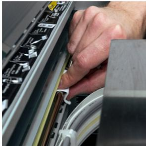
8. Once finished with cleaning, manually slide the print head to the right and into the parked position.
