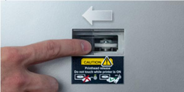
5. Press the gear slightly in and rotate counter-clockwise. As you rotate the gear, apply slight pressure to the print head with the intent of sliding it to the left. Continue to rotate the gear until the print head is freed and slide it to the left.
