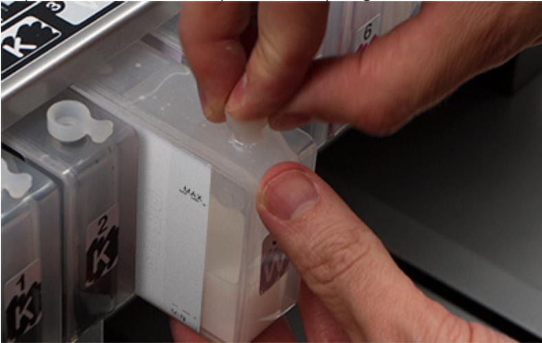
5. Shake the cartridge back and forth for a few seconds. This will ensure that the ink stays homogeneous.
