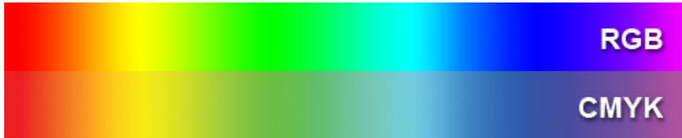
If this image were to be printed using CMYK inks, the differences in the two halves would be far less noticeable. This is why you can create an incredibly vibrant green on screen, but when it is printed, it may look darker and less brilliant.
