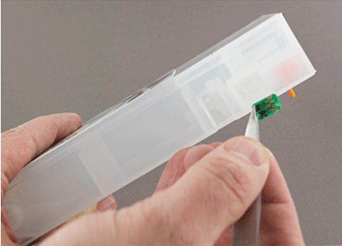
4. Attach the removable part that holds the ARC on top of the original Epson chip.
