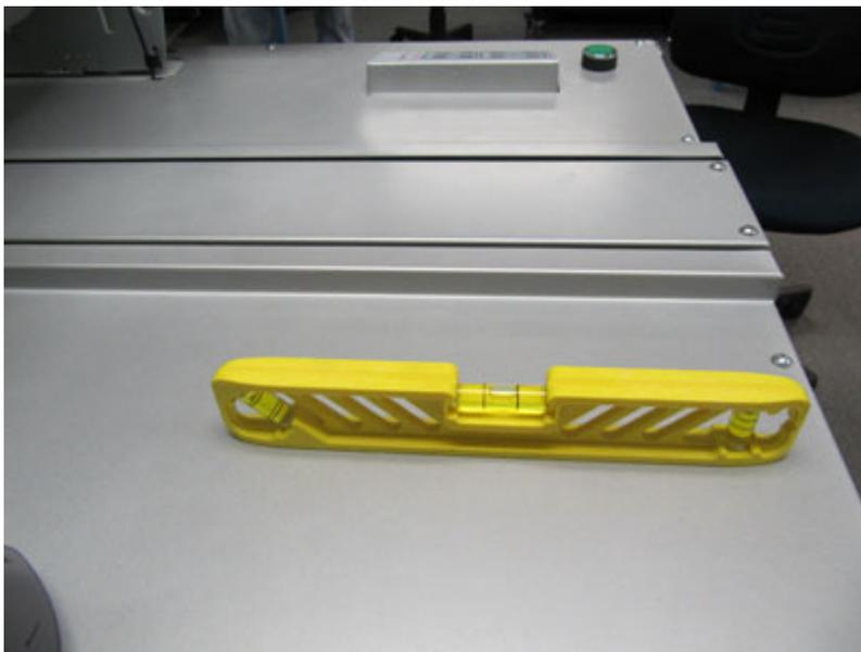
2. Check to make sure the machine is leveled left to right.
