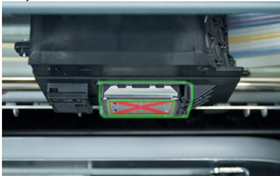
Clean only the area highlighted with green in the image. The area with the red "X" is the nozzle plate and must be avoided.
