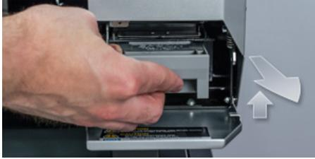
2. Empty and properly dispose of the remaining ink from the maintenance tank. Make sure to not get ink on the maintenance tank chip.
