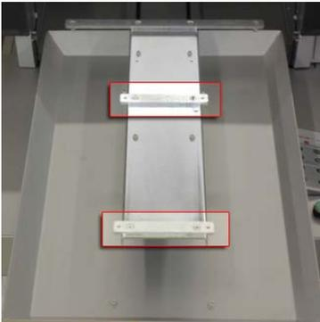
4. Align the Sleeve Table and the Adapter Plate as shown in the picture below and secure them to the Table Support using six (6) M4 Countersunk Hex Screws.
