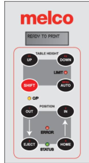
*Once the table height is adjusted for a style of garment, it shouldn't need to be adjusted until the style is changed.*
