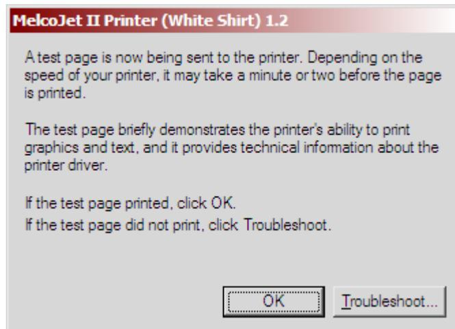
If you receive the above request to print a test page, you will need to lay down a few sheets of standard “8 ½ x 11” white paper on your print table. Be sure to completely cover the table so the Windows test print remains on the paper saving you from cleaning the table.
