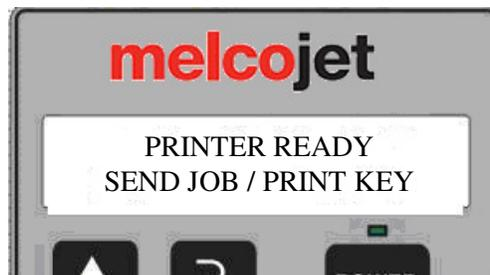
*Figure 37 message indicating complete power up of print engine*
