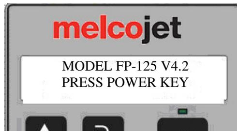
*Figure 4.1 Main power on LCD message*
